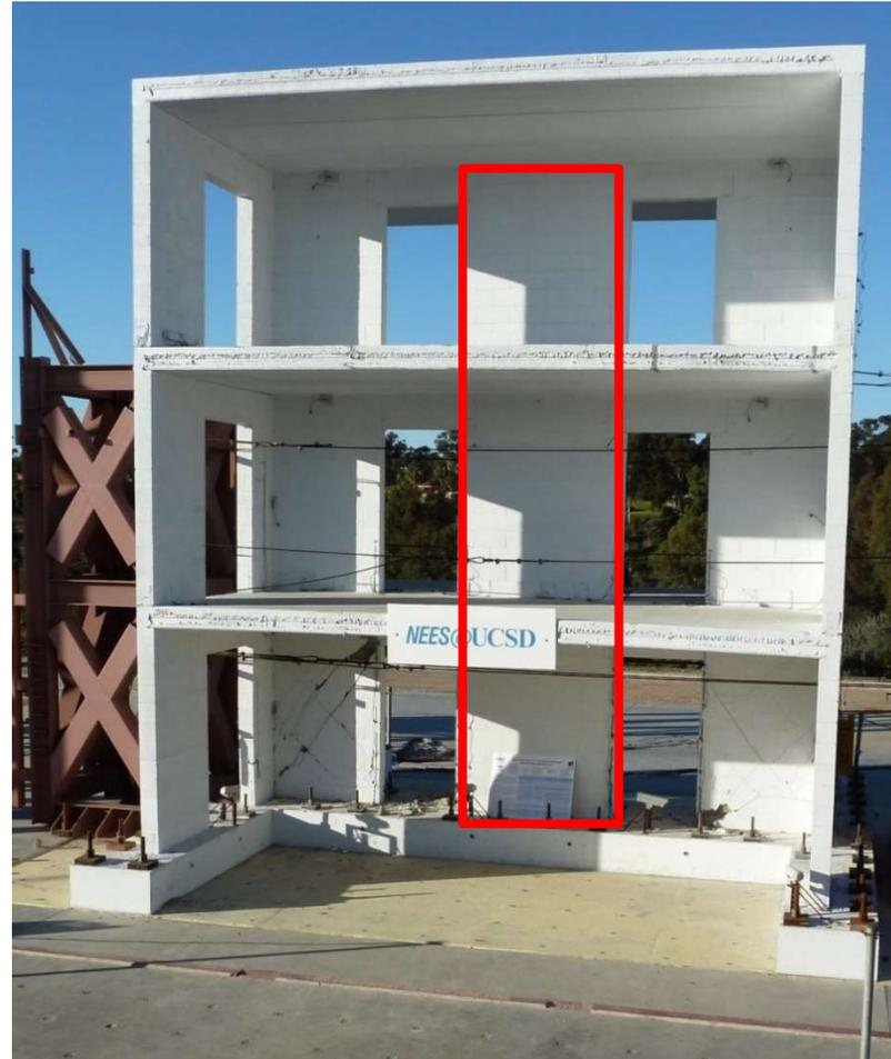
Shaking table testing of a 3-storey full-size RM building at UC San Diego, USA (Shing, Klingner, Stavridis, et al. 2011)
