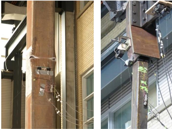
Figure 2. Failure modes of BIEs: low-cycle-fatigue-induced fracture (left) and tension fracture (right) (reproduced from [2]).
