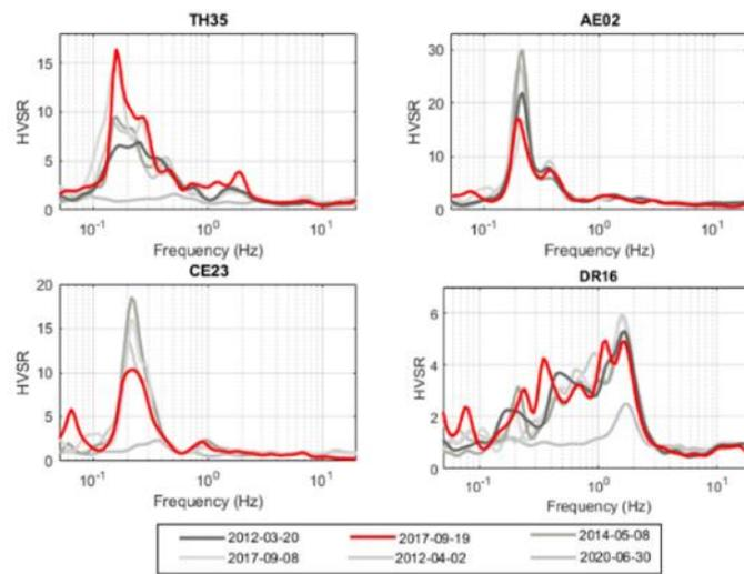
Figure 6. Earthquake HVSR spectra of weak (grey) to strong (red) earthquake recordings at 4 Mexico City seismic stations.
