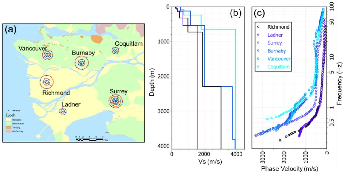
Figure 2. (a) Six large array sites in Metro Vancouver for which (b) the optimal  $V_s$  depth profile is determined from inversion of (c) fundamental-mode Rayleigh wave phase velocity dispersion curve.
