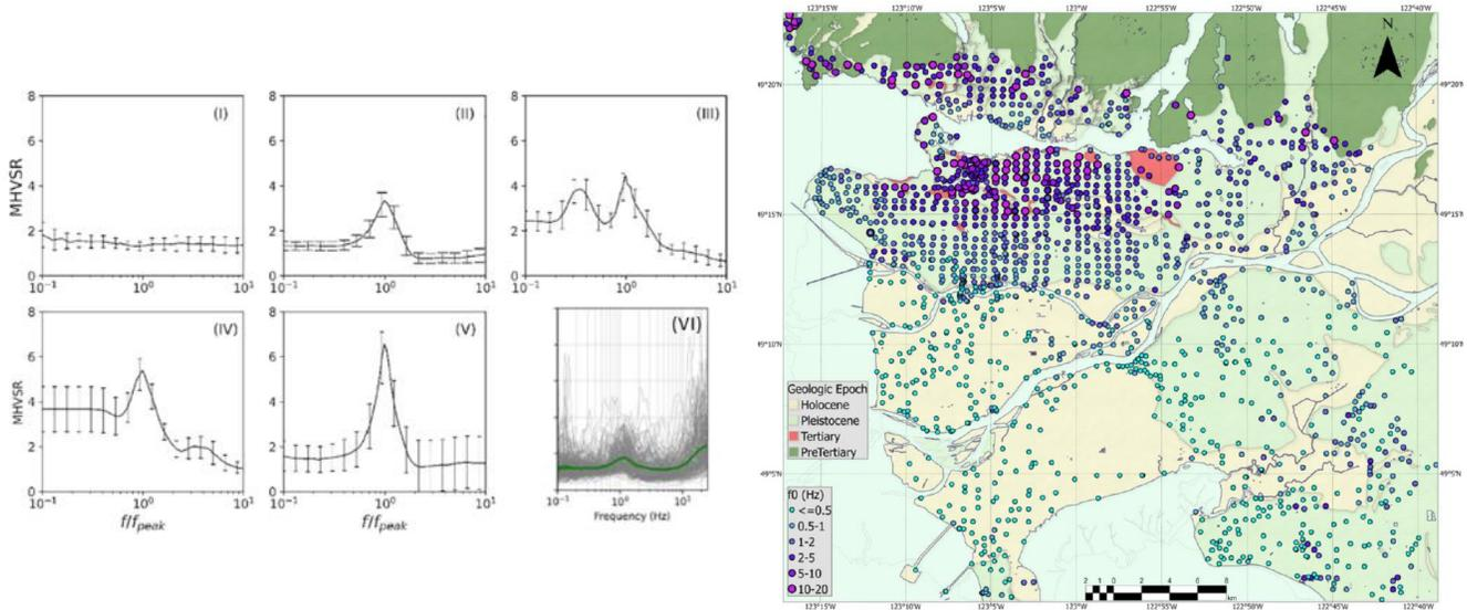
Figure 5. (left) Typical MHVSR amplification response (normalized by  $f_{0HV}$ ) within western Metro Vancouver. (right) Over 2,000 MHVSR locations (circles) depicting  $f_{0HV}$  (colouring) overlaid on a simplified surficial geologic map.
