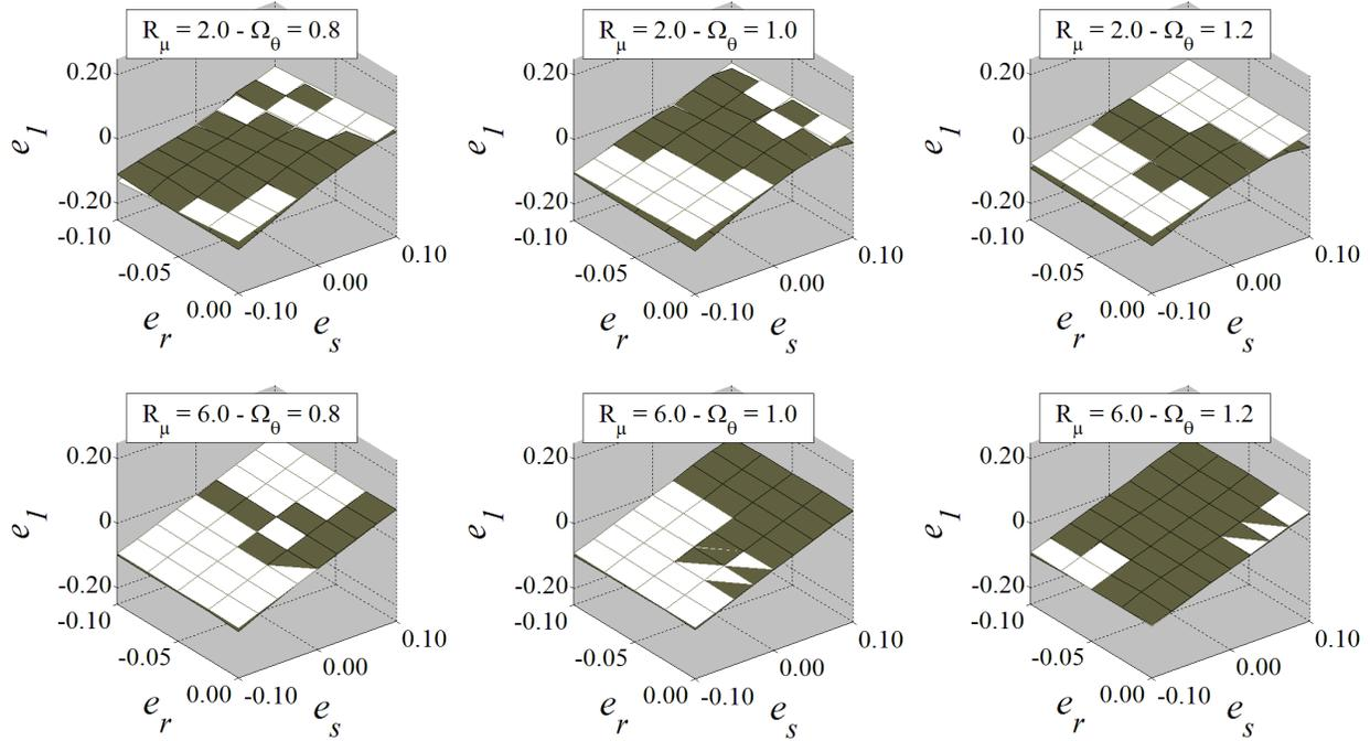
**Fig. 4 – Corrective eccentricities for side 1 (stiff side) as a function of  $e_r$  and  $e_s$**
