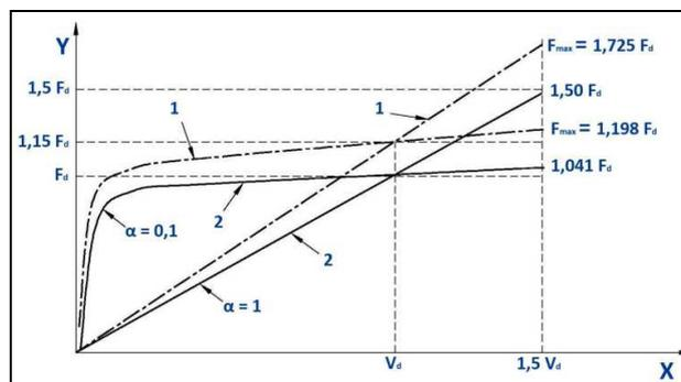
Fig. 3 – Force (Y) versus Velocity (X) curves for a linear damper ( $\alpha=1$ ) and a non-linear damper ( $\alpha=0.1$ ) – as per Equation 1
