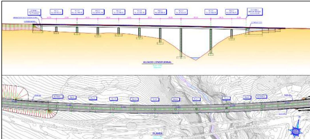
Fig. 4 – Longitudinal section and top view of the bridge over the Rio Frio, AVE Quejigares-Loja
