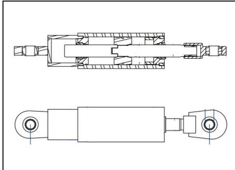
Fig. 2 –Section of a typical shock absorber (top) showing piston, and elevation (bottom)
