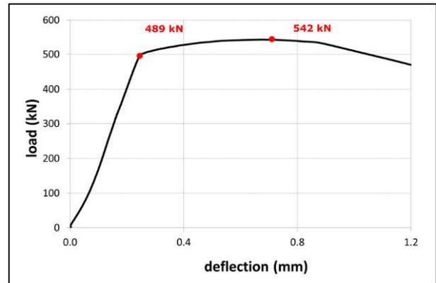
**Fig.15 – Break-Away Test – Load/Deflection curve for one of the fuse elements (#2)**
