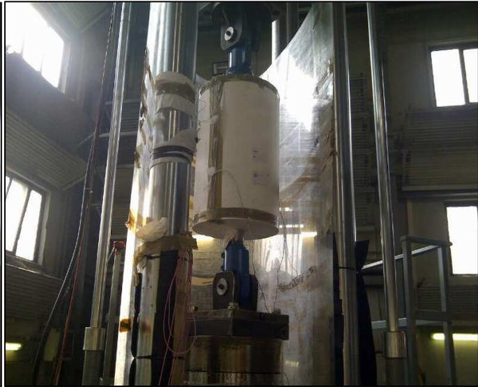
**Fig.11 – Prototype damper undergoing a low temperature test (-25°C)**
