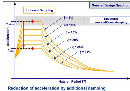
**Fig. 1 – Response spectra for a structure with increasing damping**
