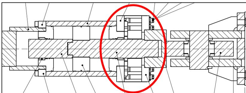
**Fig.6 – Detail of the fuse arrangement for the shock absorber**
