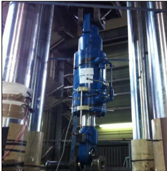
**Fig.10 – Prototype damper during testing at Politecnico di Milano, Italy**
