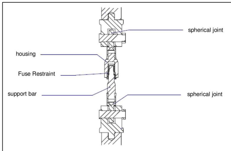
Fig.13 – The test set-up for a single fuse element
