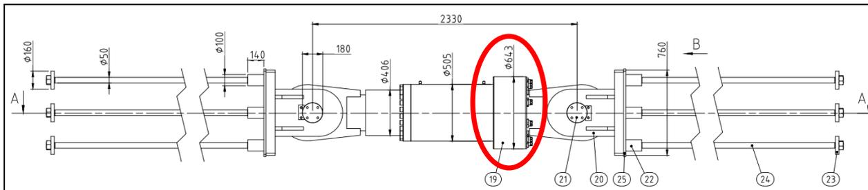
**Fig.5 – Elevation of the Reston-SA shock absorber with concrete anchors and fuse**
