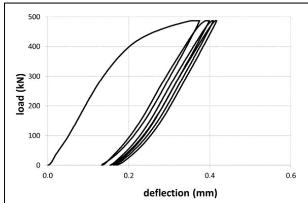
**Fig.14 – Service Load Test - Curve Load - Deflection for one of the fuse elements (#2)**
