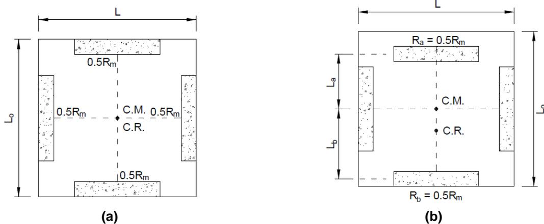
**Fig. 3 – (a) Symmetric Plan Geometry and (b) Typical Geometric Eccentricity**
