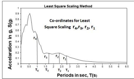
Fig. 4 Ordinates on the input GMR spectrum
