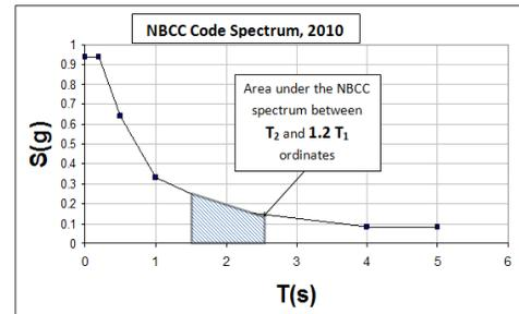
Fig. 7 P.A. under the NBCC 2010 Spectrum
