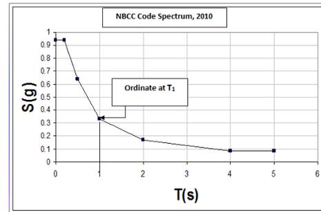
Fig. 3 Ordinate at  $T_1$  on the NBCC 2010 Spectrum
