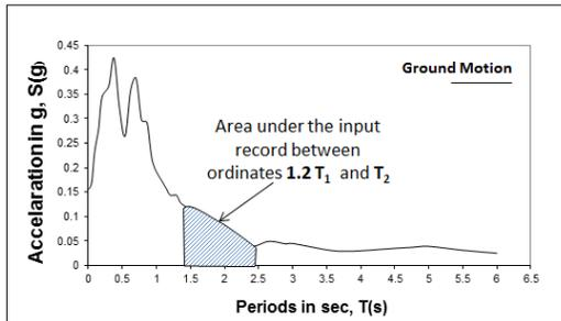
Fig. 6 Partial Area (P.A.) under the input spectrum
