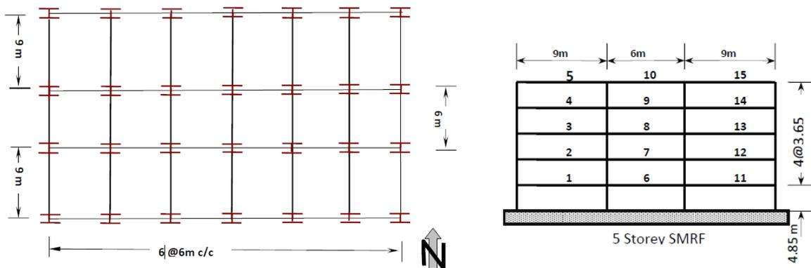
Fig. 1: Plan and elevation of the five-storey frame building
