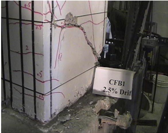
a) Immediately after shear failure
