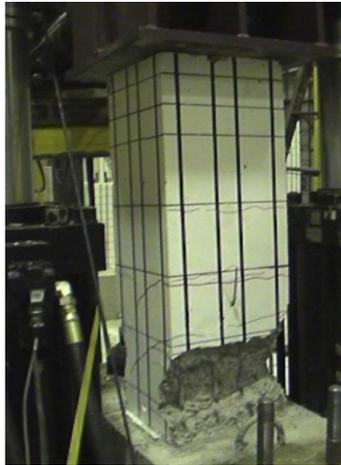
a) Concrete crushing
