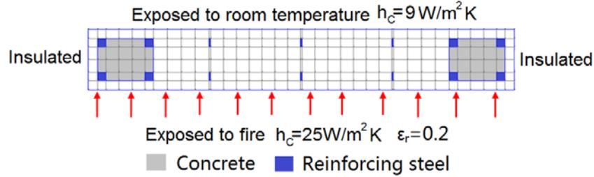
**Fig. 1 – Thermal boundary conditions of walls in SAFIR**
