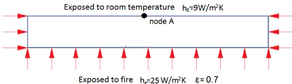
**Fig. 3 – Thermal boundary condition**
