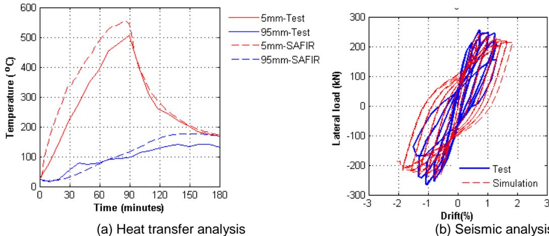
**Fig. 2 – Comparison of experimental and numerical response of wall N4T9 under fire and reversed-cyclic loading (Liu, 2010)**
