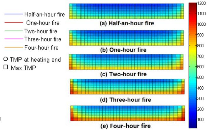
Fig. 5 – Maximum temperature of WR20 section
