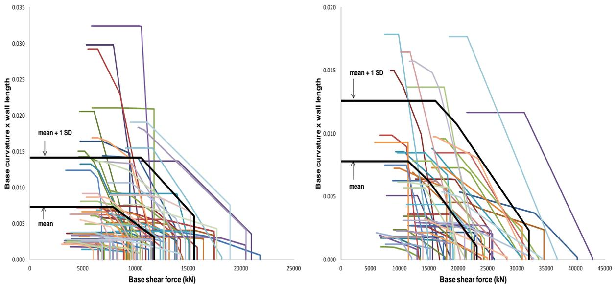
Fig. 6 – Interaction between base curvature and base shear force in: 10-story shear wall building (left); 30-story shear wall building (right).
