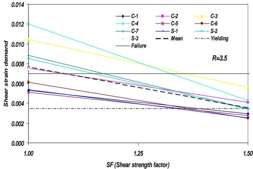
Fig. 4 – Influence of shear strength (amplification) factor used to design the horizontal reinforcement on the maximum shear strains; from Rad (2009).
