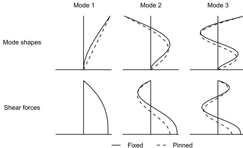
Fig. 2 – Mode shapes and shear force envelopes for fixed-based and pinned-based cantilevers.
