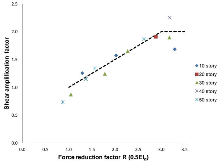
Fig. 3 – Shear amplification factors determined from NLRHA of thirteen shear wall buildings.
