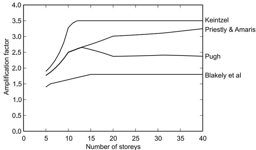
**Fig. 1** – Comparison of results from four different methods for determining shear amplification factor for case where elastic shear force demand has been reduced using a ductility force-reduction factor of 3.5.
