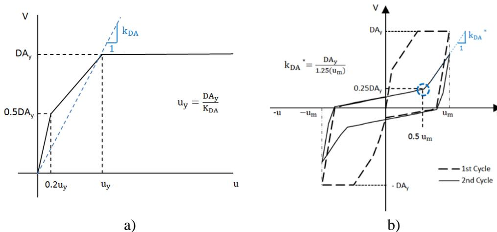
Fig. 3 – Modeling of Dowel Action Force Deformation Behavior: a) Monotonic Envelope, and b) Hysteretic Rules
