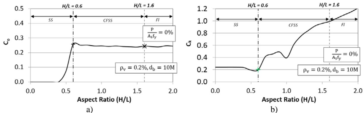
**Fig. 7 – Cyclic response of RM shear walls with low axial stress and vertical reinforcement ratio of 0.2% at  $\mu=2$ : a)  $C_o$  vs H/L ratio, and b)  $C_k$  vs H/L ratio.**
