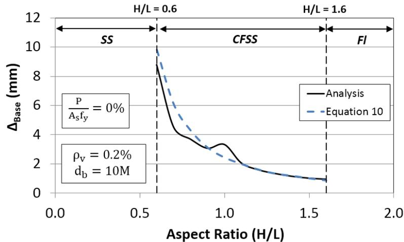
**Fig. 8 – Sliding displacements in RM shear walls with low axial stresses and vertical reinforcement ratio of 0.2% at a  $\mu$  value of 2.**
