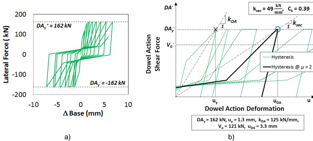
**Fig. 6 – Cyclic response of an RM shear wall with H/L ratio of 1.0 experiencing CFSS mechanism: a) Dowel action hysteresis, and b) Estimation of dowel action secant stiffness,  $k_{sec}$ , at  $\mu$  value of 2.**
