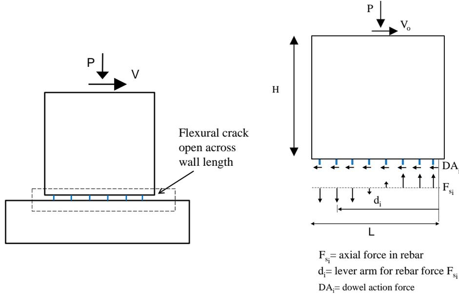
**Fig. 5 – Lateral resistance of an RM shear wall with open flexural crack: a) Wall loading and cracked at wall-foundation interface, and b) Vertical reinforcement resisting external loading through dowel action, DA, and axial forces,  $F_s$ .**
