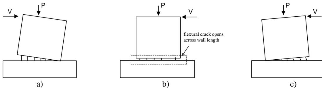
**Fig. 1 - Sliding Shear in Combination with Flexural Yielding in RM Shear Walls: a) Flexural Yielding Occurs; B) Loading Direction Changes, and Sliding Starts at the Base, and C) Shear Force Transferred to the Base Through Dowel Action until a Flexural Crack is Closed**
