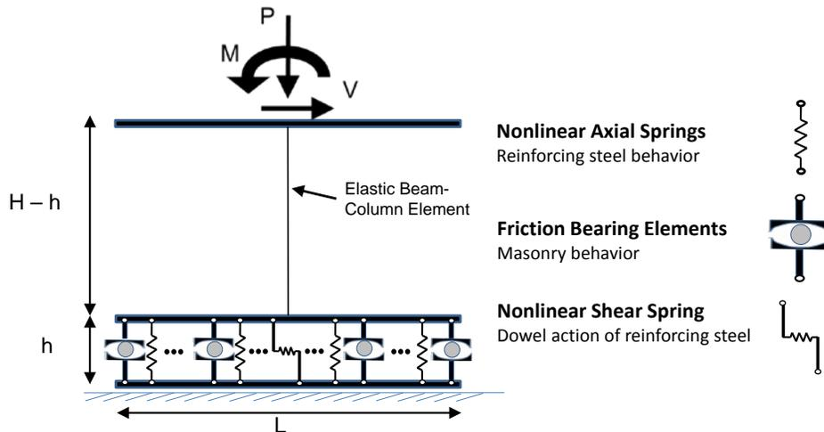
Fig. 2 - RM Cantilever Wall Model
