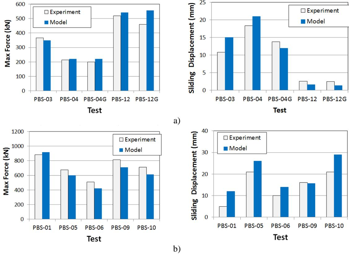
Fig. 4 – A Comparison of Peak Forces and Displacements From Calibrated Analysis Model vs Experimental Results: a) Cantilever Walls, and b) Fixed-Fixed Walls
