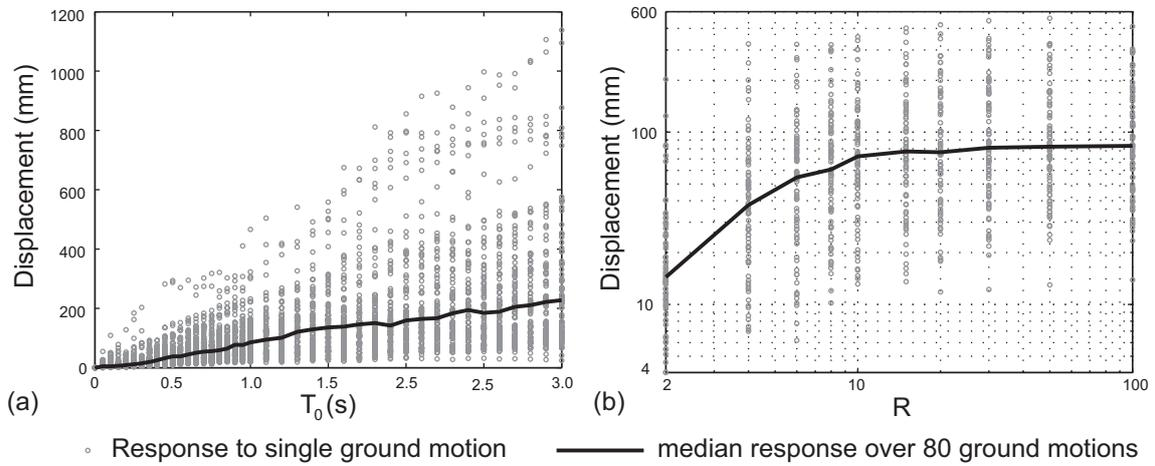
**Fig. 3 – Displacement affected by (a) initial period and ground motion when  $R = 2, T_{\tan} = \infty, \beta = 0.4$  and (b) linear limit and ground motion when  $T_0 = 0.3\text{s}, T_{\tan} = \infty, \beta = 0.4$**
