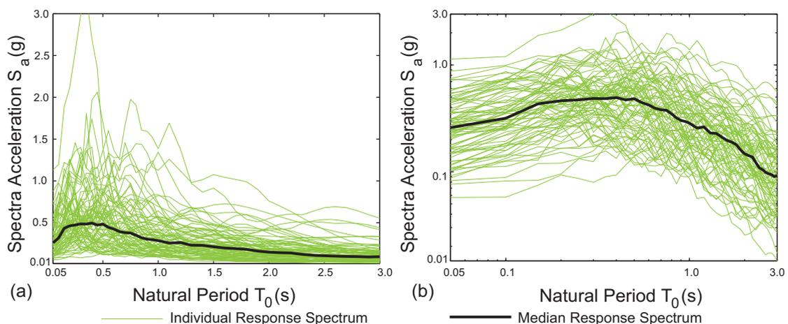
**Fig. 2 – Elastic response spectra of ground motions considered:**
