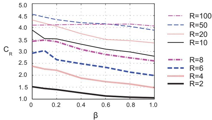
Fig. 5 – Effect of  $\beta$  on median  $C_R$  for  $T_0 = 0.5\text{s}, T_{\tan} = \infty$
