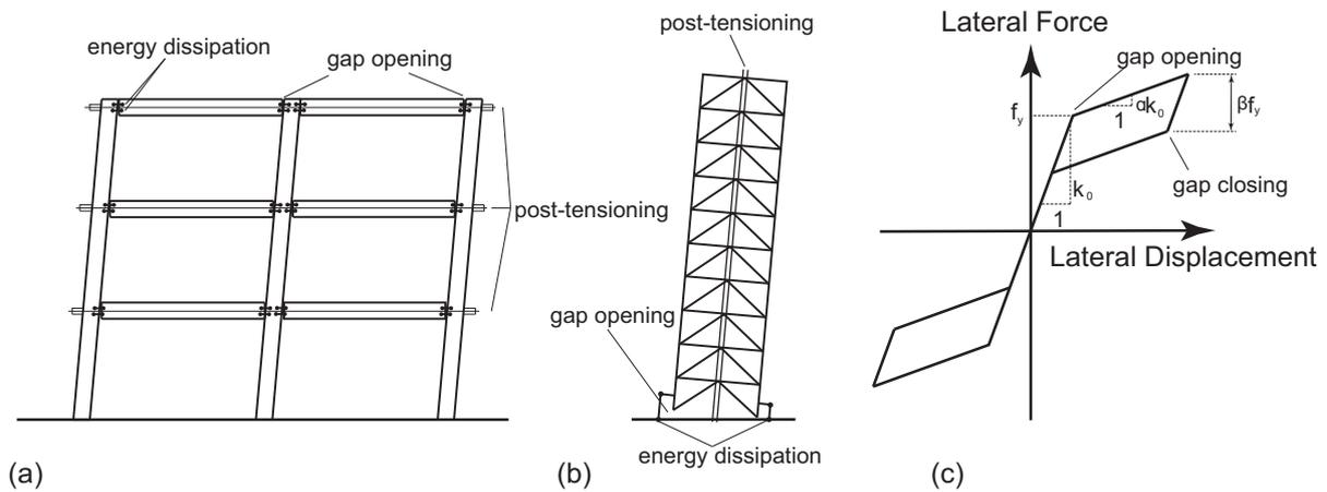
**Fig. 1 – (a) Self-centering moment resisting frame; (b) controlled rocking steel braced frame; (c) flag-shaped hysteresis**
