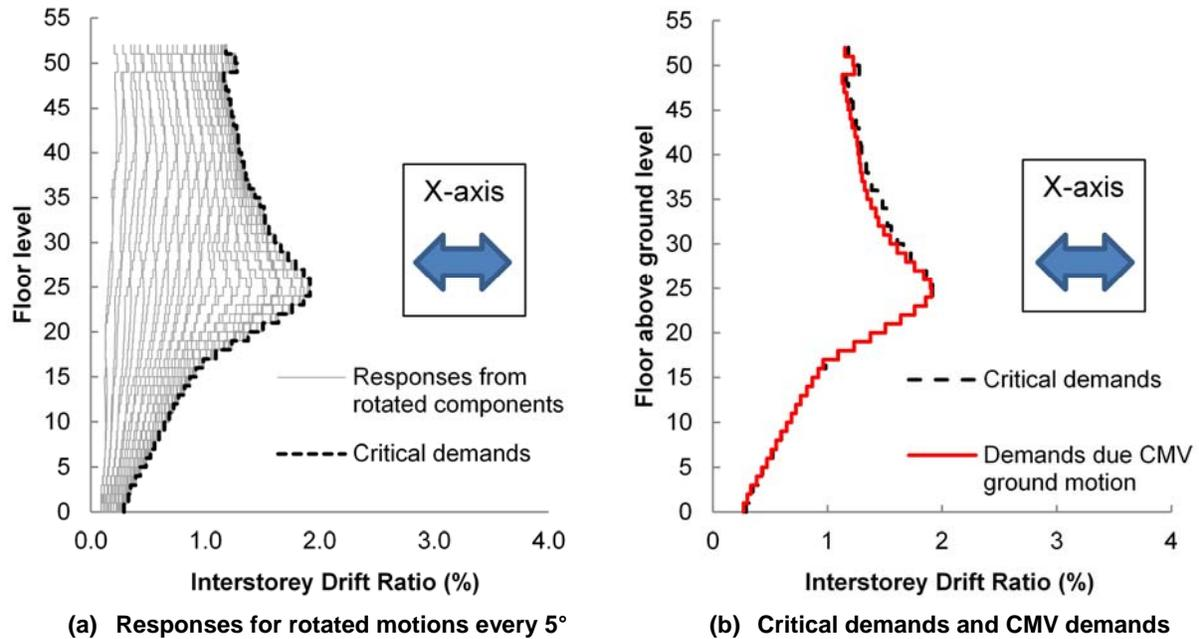
**Fig. 6 – Prediction of critical interstorey drift ratio demands in the X-direction**
