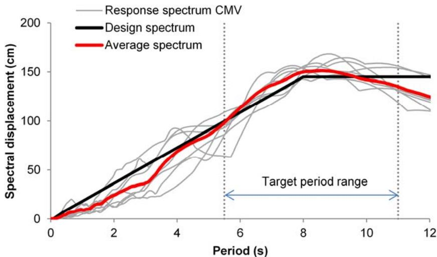
**Fig. 4 – Design spectrum and spectra for CMV input motions of suite 2 in the Y-direction**
