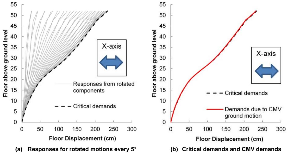
**Fig. 5 – Prediction of critical displacement demands in the X-direction**
