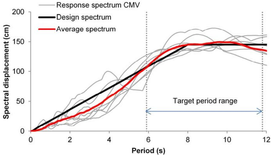
**Fig. 3 – Design spectrum and spectra for CMV input motions of suite 1 in the X-direction**
