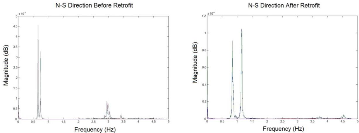
**Fig. 3 – Sample Power Spectral Density Plot for One Test Setup Before and After Retrofit**
