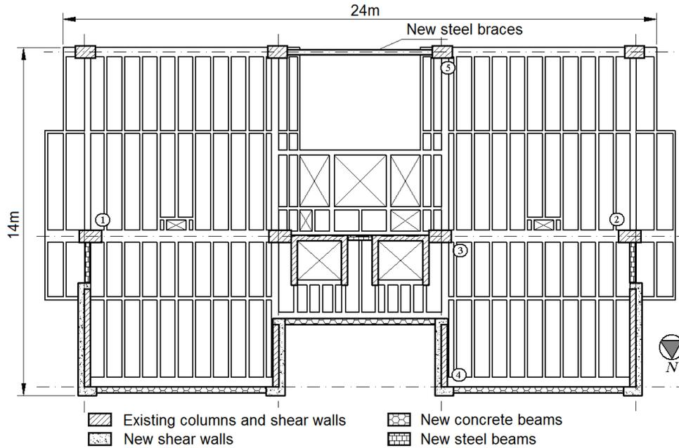
**Fig. 1 – Buildings 1A and 1B: Existing LLRS, Retrofit Solution and Sensor Location**
