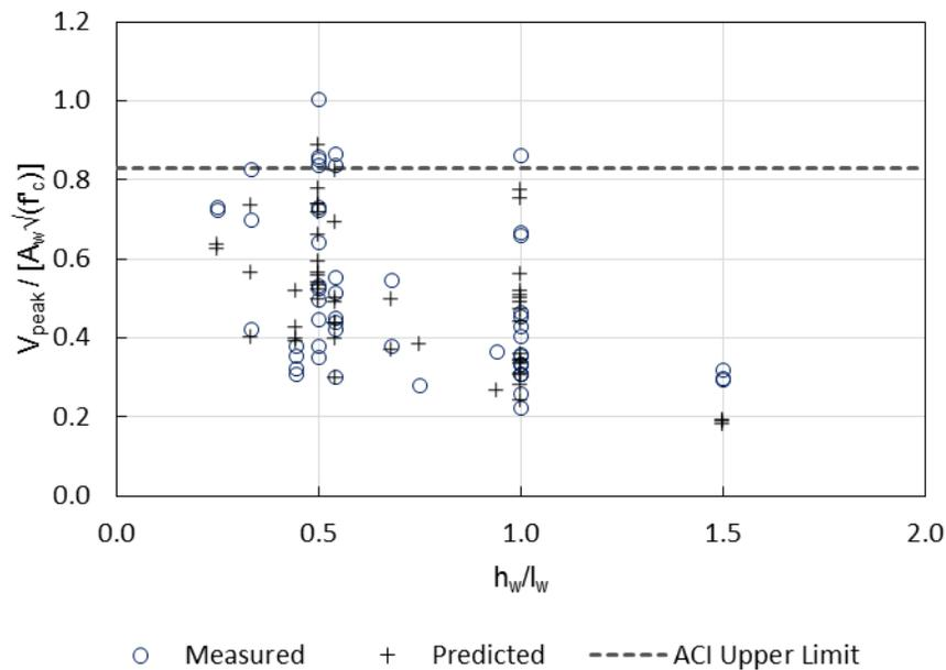
**Fig. 3 – Variation of the Predicted and Measured Normalized Peak Shear Strength with Wall Aspect Ratio Compared to ACI 318 Upper Limit**
