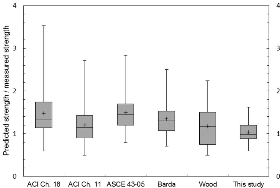
**Fig. 2 – Distribution of the Ratio of Predicted to Measured Peak Strength**
