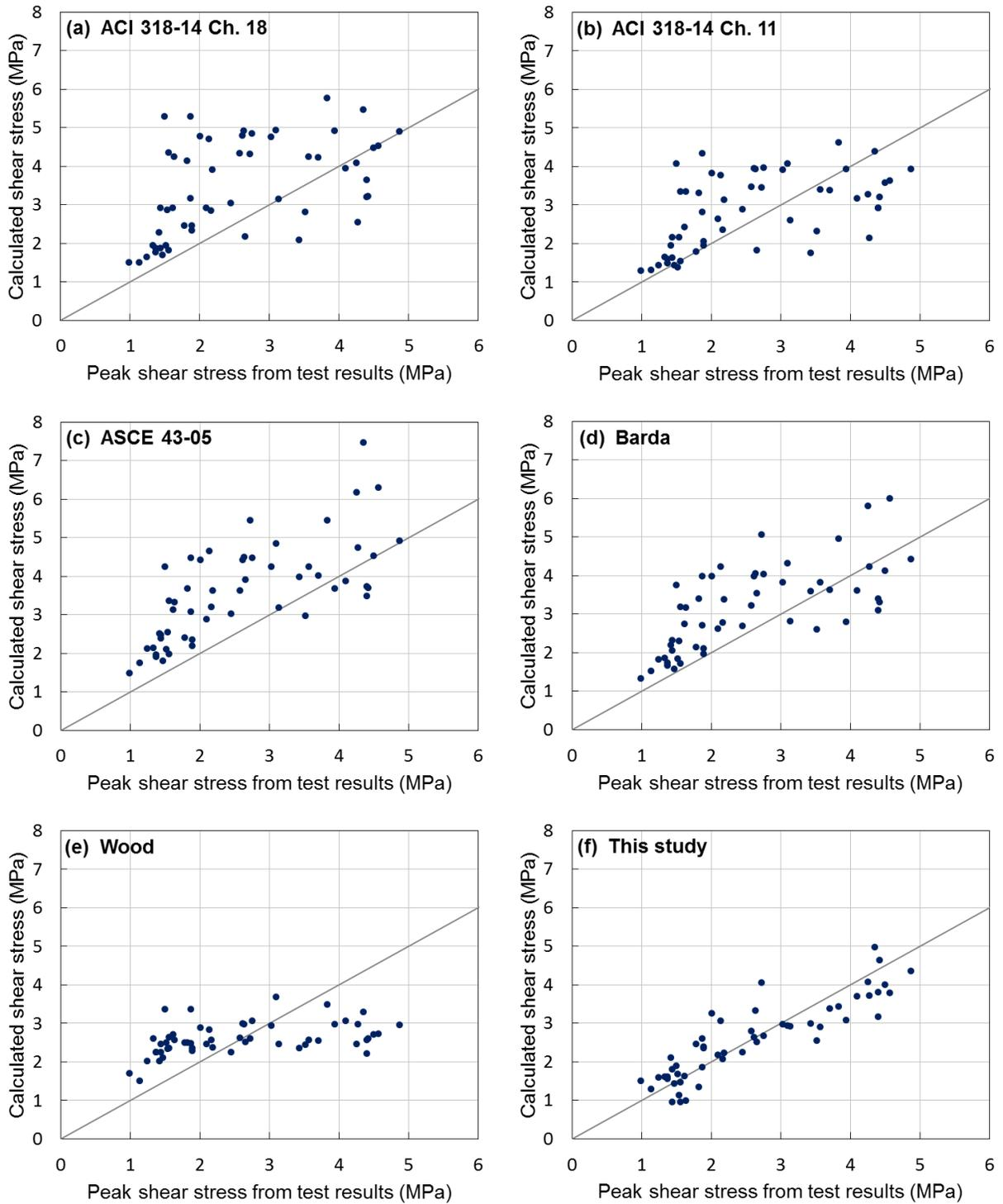
**Fig. 1 – Correlation Between Calculated Nominal Shear Stress and Measured Peak Shear Stress Using Various Available Equations: (a) to (e); and the Equation Proposed in this Study (f)**
