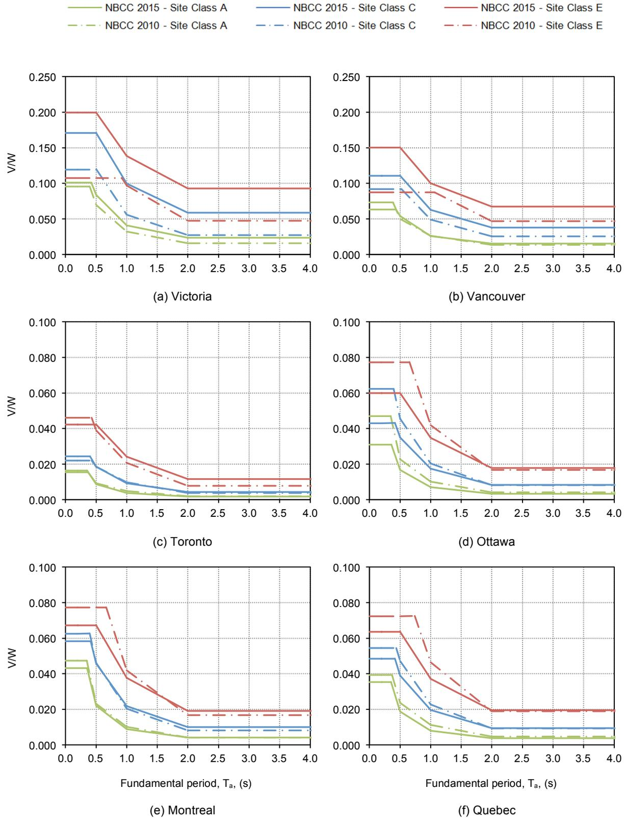
**Fig. 2 – Comparison of 2010 NBCC and 2015 NBCC V/W Ratios for Concrete Ductile Moment-Resisting Frame SFRS For Site Class A, C and E**
