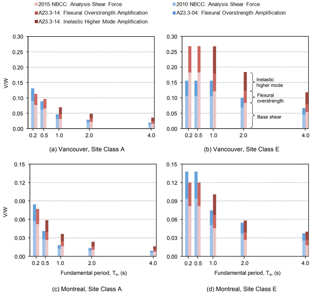
**Fig. 4 – Comparison of Design  $V/W$  Ratios for Concrete Ductile Shear Walls For Site Classes A and E**
