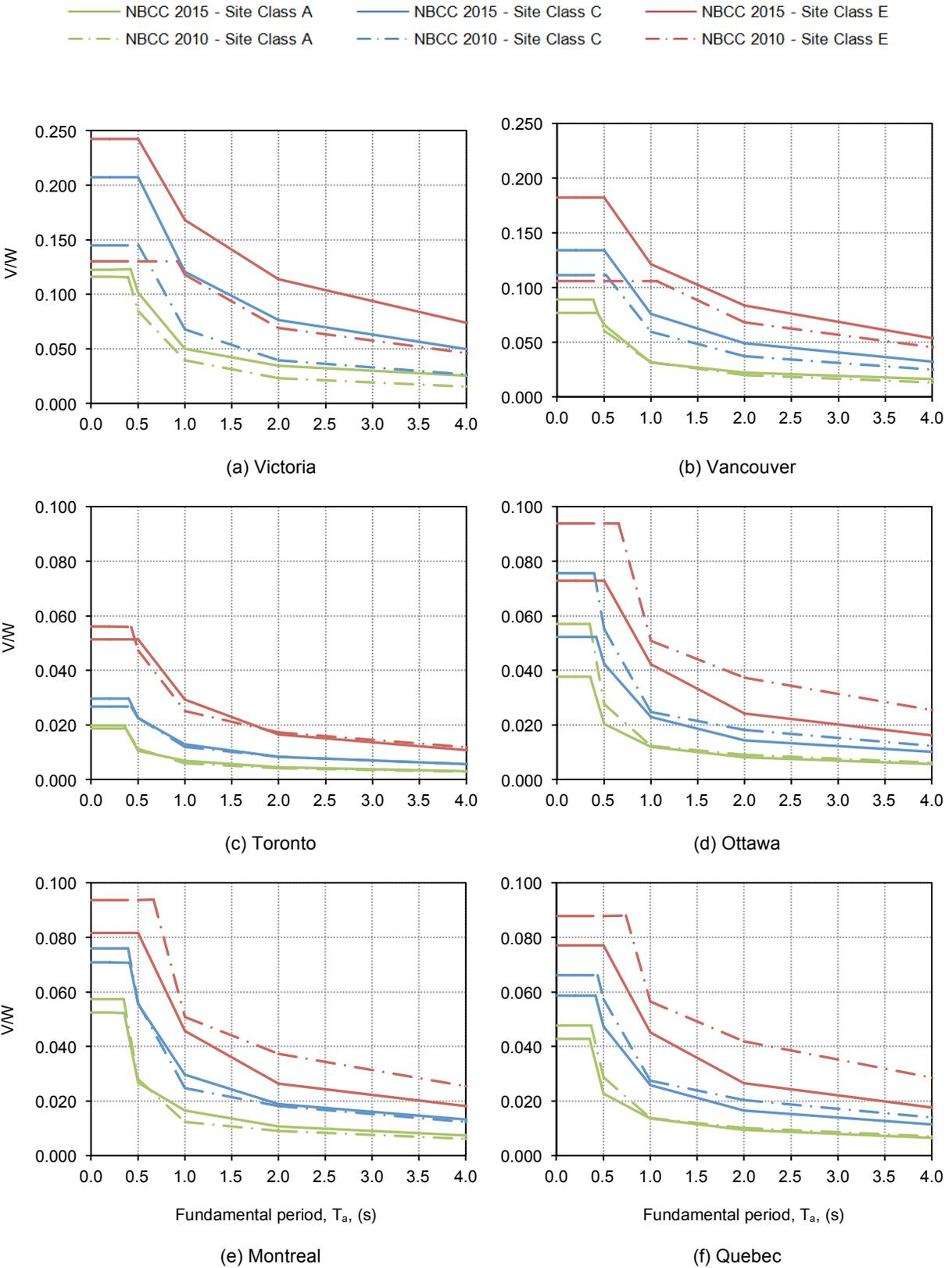
**Fig. 1 – Comparison of 2010 NBCC and 2015 NBCC V/W Ratios for Concrete Ductile Shear wall SFRS For Site Class A, C and E**
