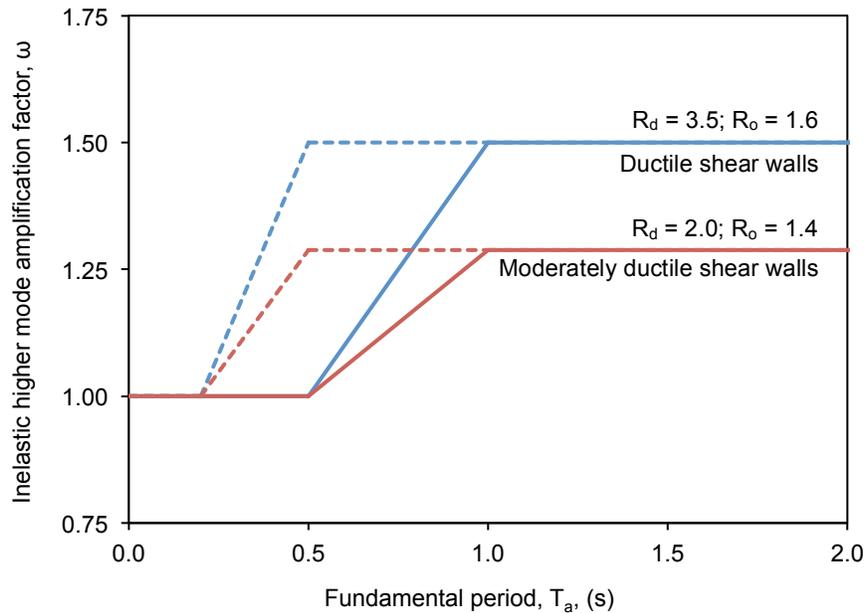
**Fig. 3 – Inelastic higher mode shear amplification factor,  $\omega$**
