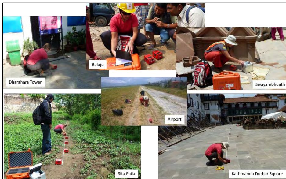
Figure 2.4: Photos of microtremor measurements performed in and around Kathmandu using ultra-portable TROMINO® sensors (small red sensors)
