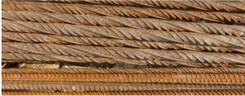
Figure 5.4: Steel reinforcing bars used for RC construction in Nepal: Torkari steel (top) and TOR steel (bottom) (Photo: Svetlana Brzev)
