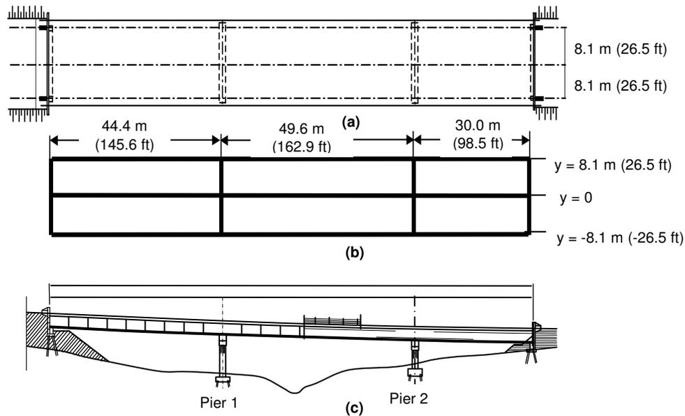
Figure 2. (a) Plan of Portage Creek Bridge, (b) Simplified Bridge Geometry, and (c) Elevation.
