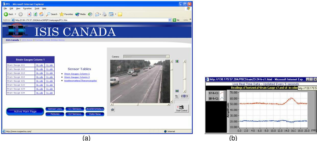
Figure 5. (a) Web-interactive page for online monitoring of the Portage Creek Birdge, (b) a typical output from a strain gauge installed in the bridge columns.
