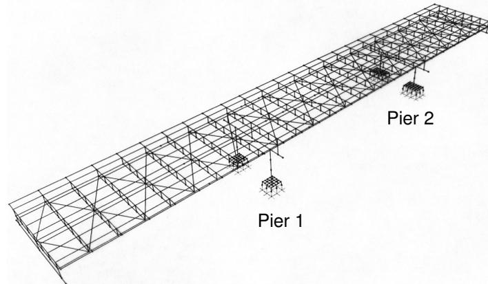
Figure 4. Finite element model of the Portage Creek Bridge.
