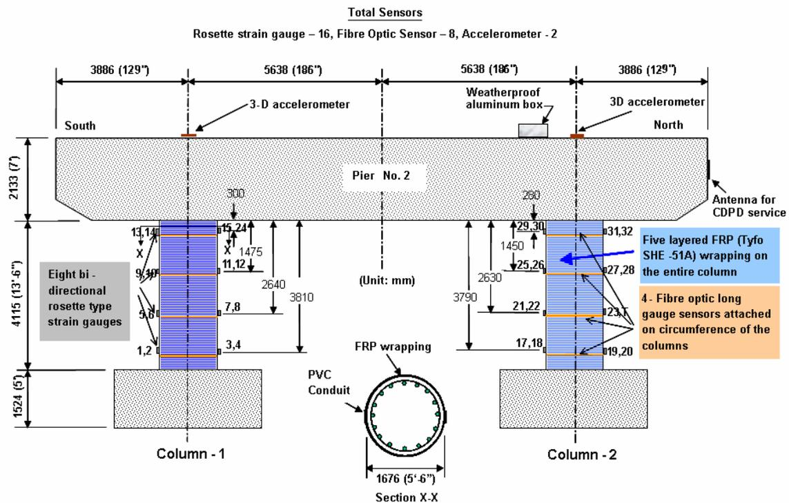
Figure 3. Elevation of Pier No. 2 (short columns) with sensor locations.
