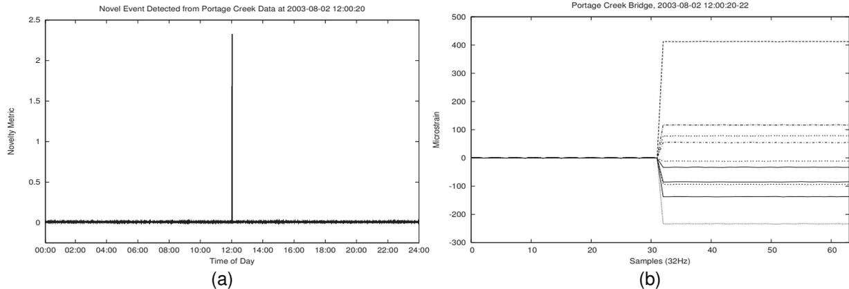
Figure 8. Novelty event detection in Portage Creek Bridge SHM System, (a) novelty metric, and (b) sensor data corresponding to the novelty event.
