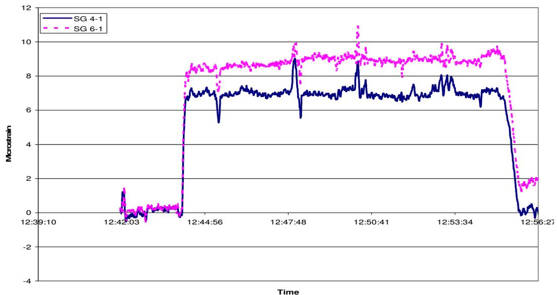
Figure 6. Increase in strain in Column 2 during the static load test.
