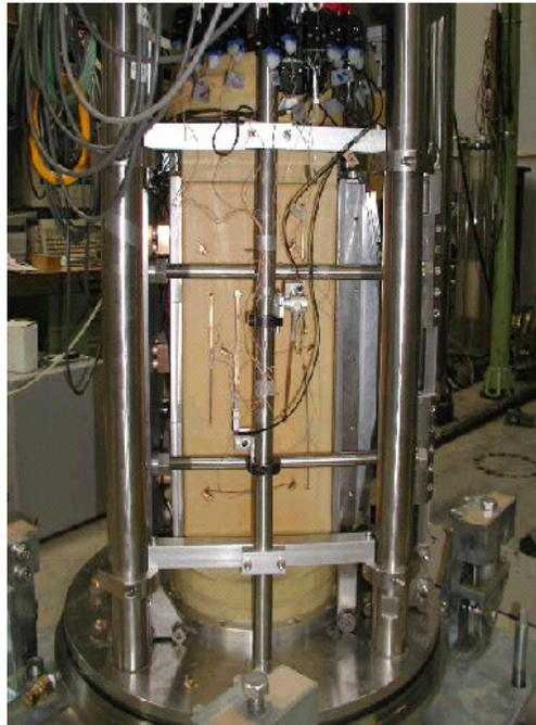
Figure 3. Prepared specimen of Chiba gravel for plane strain testing.
