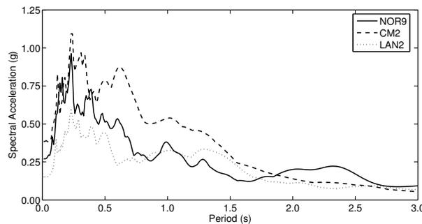
Figure 7. Acceleration spectra of considered earthquakes
