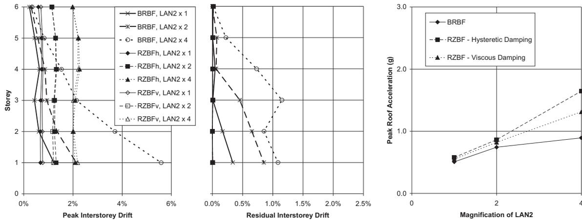
Figure 10. Peak interstorey-drifts, residual interstorey-drifts, and peak roof accelerations of test structures subjected to three magnifications of LAN2 ground acceleration record.
