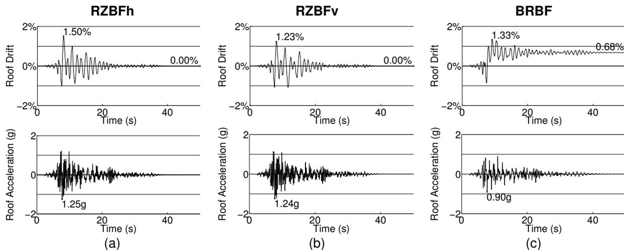
Figure 8. Time-history roof drift and acceleration response to record CM2 with magnification of 2 for: (a) rocking zipper-braced frame with hysteretic damping; (b) rocking zipper-braced frame with viscous damping; (c) buckling-restrained braced frame
