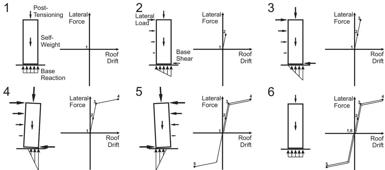
Figure 1. Schematic response of a base-rocking structure.
