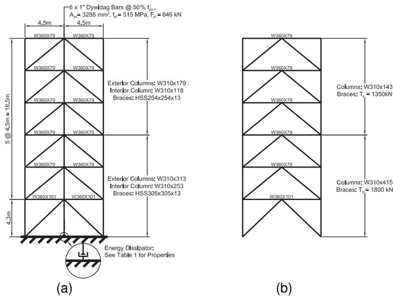
Figure 5. Designs of (a) rocking zipper-braced frame; (b) buckling-restrained braced frame.
