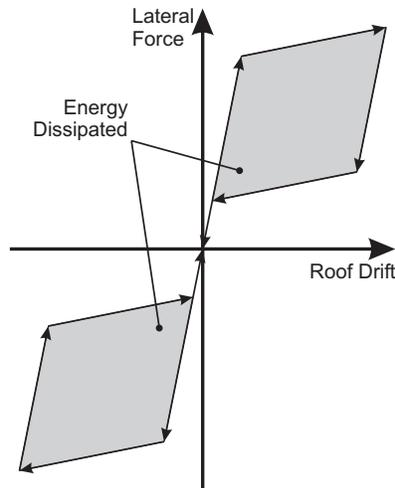
Figure 2. Schematic response of a base-rocking structure with hysteretic damping.
