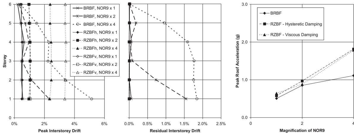
Figure 11. Peak interstorey-drifts, residual interstorey-drifts, and peak roof accelerations of test structures subjected to three magnifications of NOR9 ground acceleration record.
