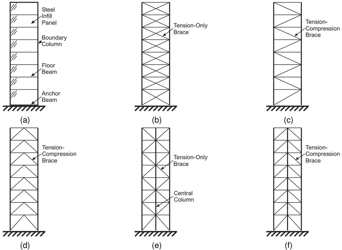
Figure 3. Schematic drawings of considered base-rocking systems: (a) steel plate shear wall; (b) vertical truss with tension-only braces; (c) vertical truss with tension-compression braces; (d) chevron-braced frame; (e) two-storey X-braced frame; (f) zipper-braced frame
