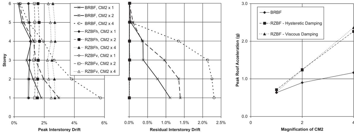
Figure 9. Peak interstorey-drifts, residual interstorey-drifts, and peak roof accelerations of test structures subjected to three magnifications of CM2 ground acceleration record.
