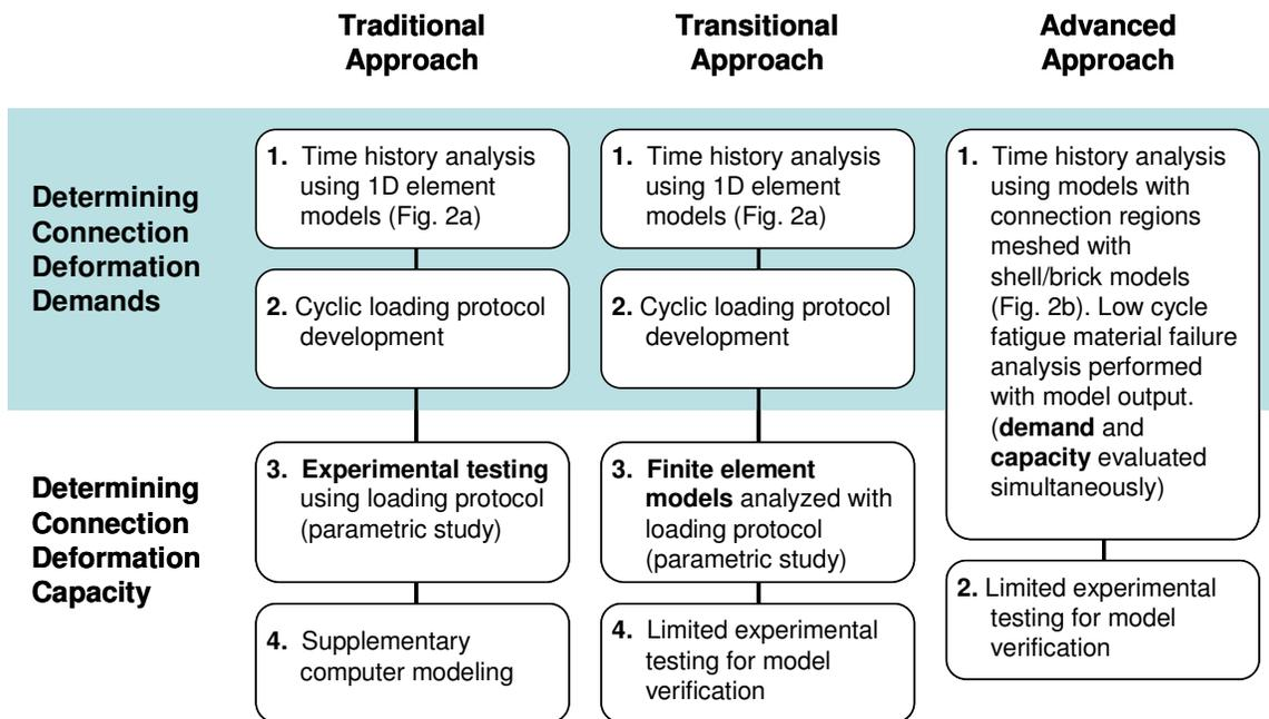
Figure 1. Procedures for verifying connection performance under seismic loading.
