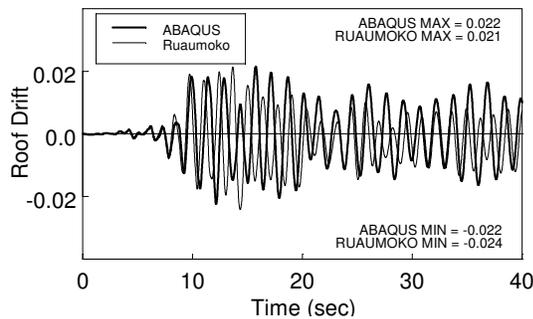
Figure 13. Roof drift under 1xrecord.
