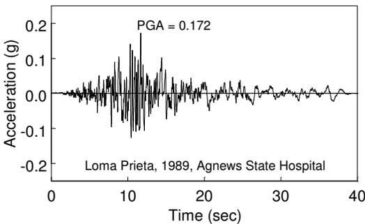
Figure 9. Earthquake record used for analyses.
