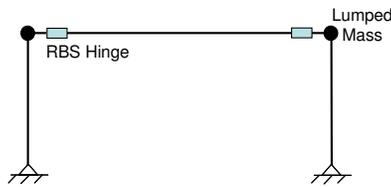
Figure 7. 1D Model with Plastic Hinges.
