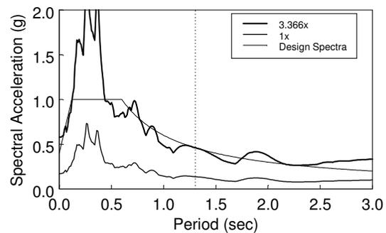
Figure 10. Spectra for 1x and 3.366x events.
