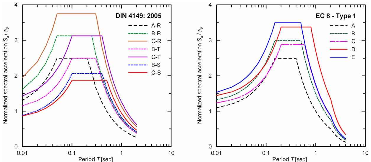
Figure 2. Normalized elastic design spectra (damping  $\xi = 5\%$ ) for site classes of the earthquake code provisions (a) DIN 4149:2005 (NABau, 2005) and (b) Eurocode 8 – Type 1 (CEN, 2002).
