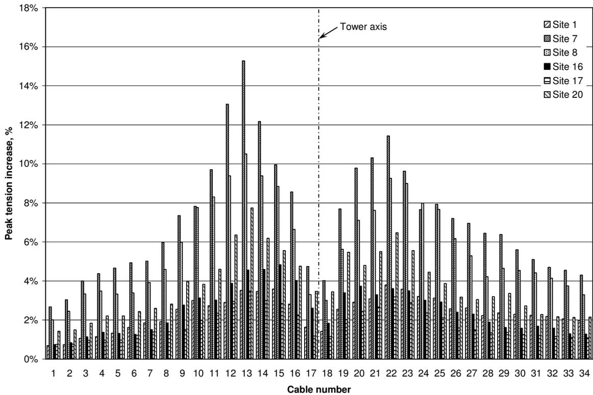
Figure 8. 3D Seismic response of bridge 3 for the six Saguenay sites used.
