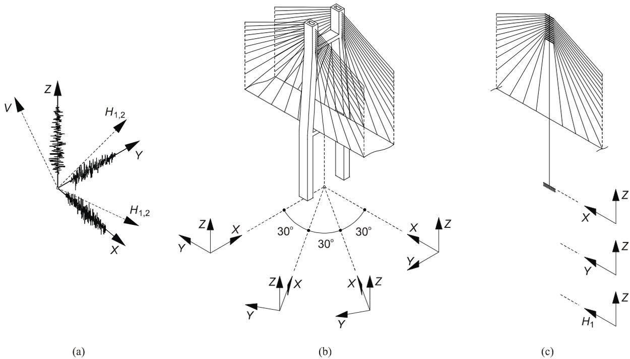
Figure 4. Presentation of the seismic input: a) Principal direction; b) 3D seismic input; c) 2D seismic input.
