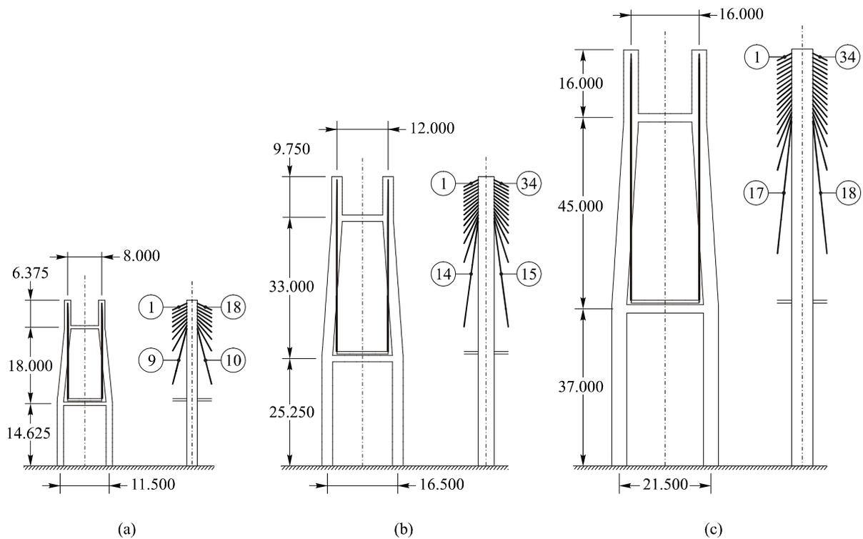
Figure 2. Elevations of the pylons and numbering of the stay cables for the three bridge models studied: (a) Bridge 1, (b) Bridge 2, and (c) Bridge 3 (dimensions in meters).
