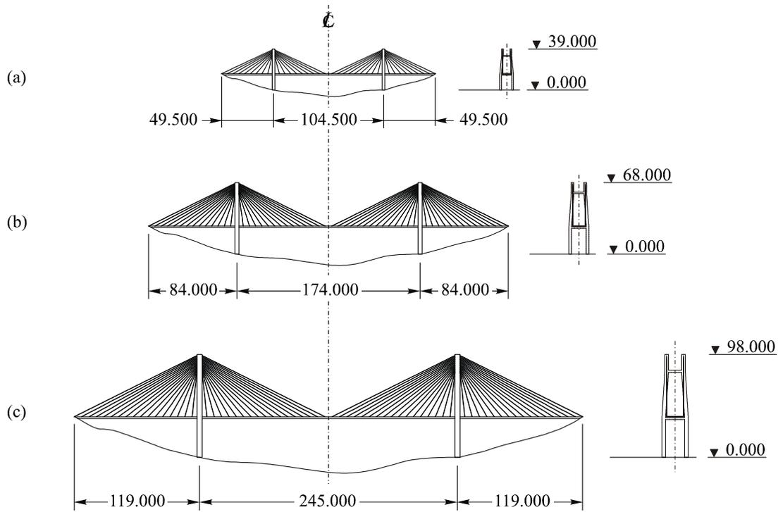
Figure 1. Elevations of the three bridge models studied (dimensions in meters).
