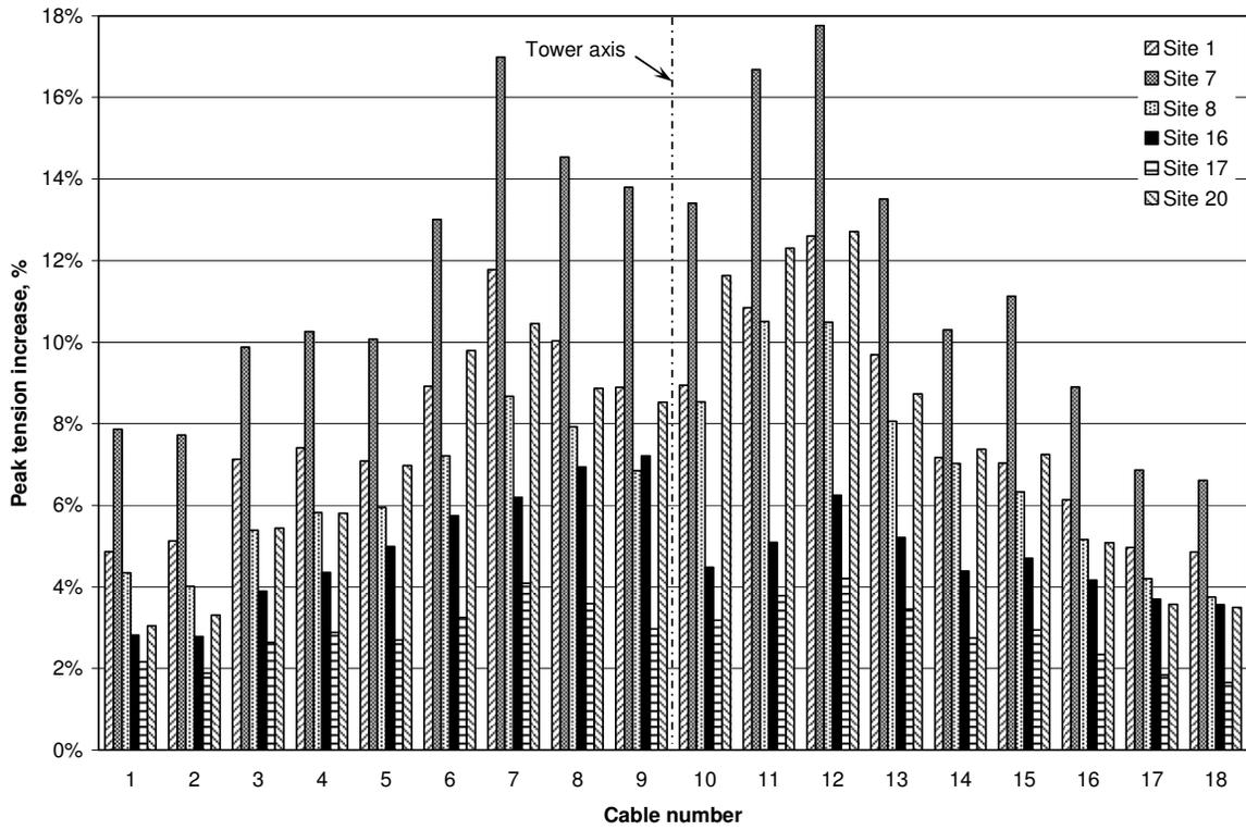
Figure 6. 3D Seismic response of bridge 1 for the six Saguenay sites used.
