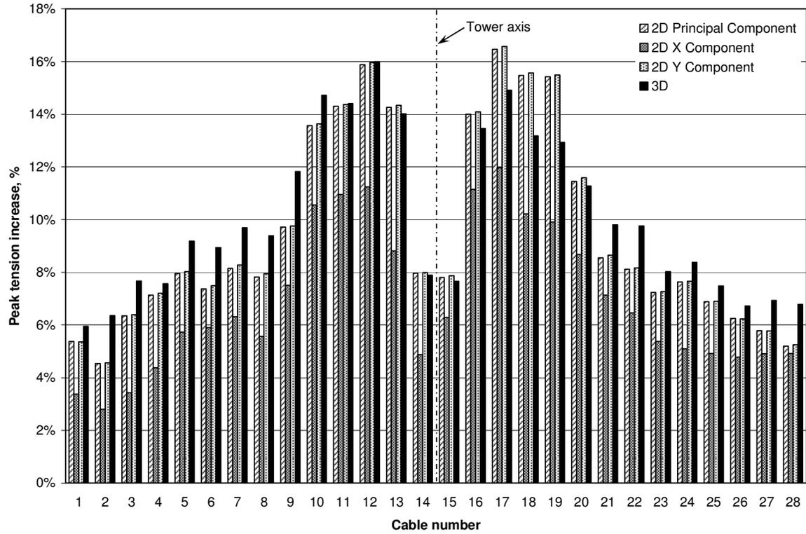
Figure 11. 2D vs 3D seismic analysis - Bridge 2 - Site 7.
