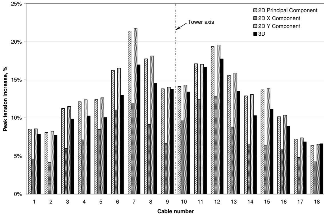
Figure 9. 2D vs 3D seismic analysis - Bridge 1 - Site 7.
