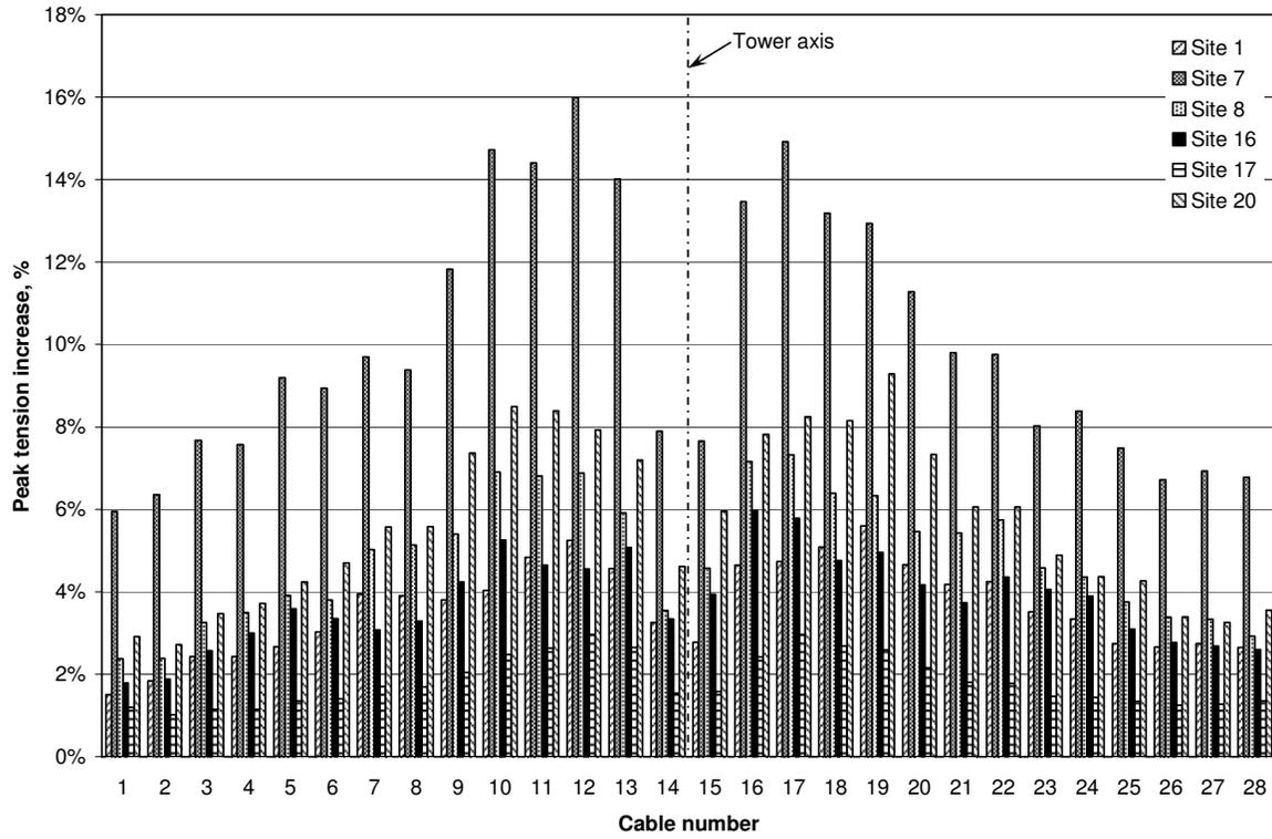
Figure 7. 3D Seismic response of bridge 2 for the six Saguenay sites used.
