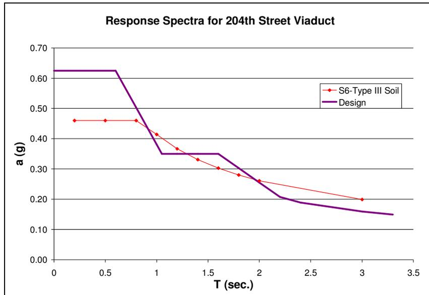
Figure 4. Design spectra for the 204<sup>th</sup> Street Viaduct project.
