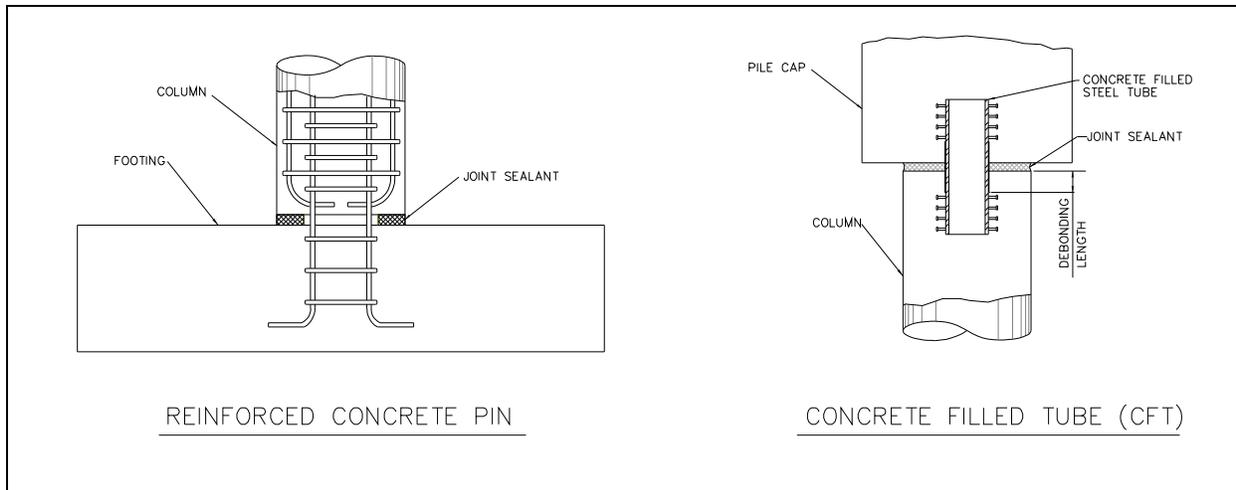
Figure 1. Two types of column pins.
