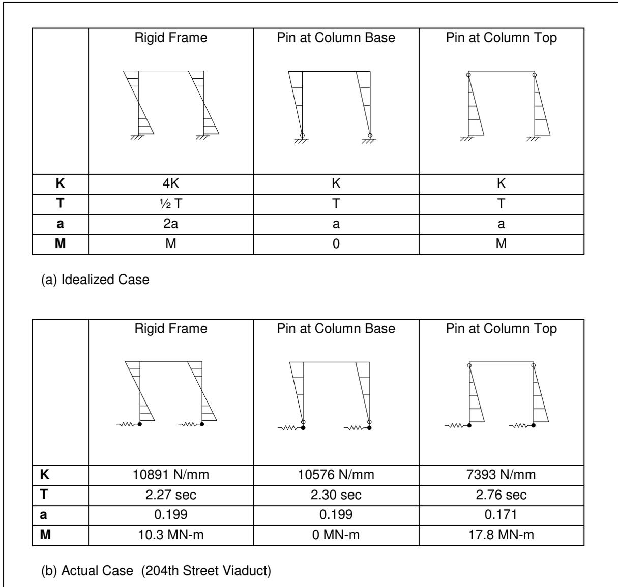
Figure 5. Frame analysis for idealized case and actual case.
