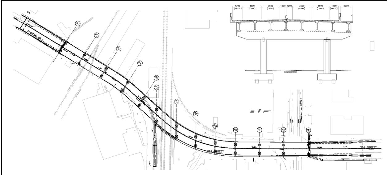
Figure 2. Overall plan and typical bent cross-section for the 204<sup>th</sup> Street Viaduct.
