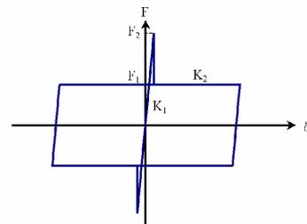
Figure 3. Restoring force model of non-linear behavior of fixed bearing model.
