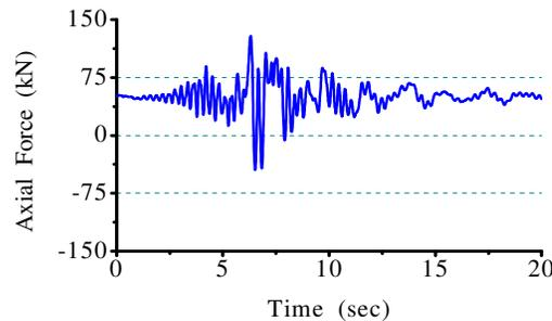
Figure 7. Time history of axial force at bearing (Case-1).
