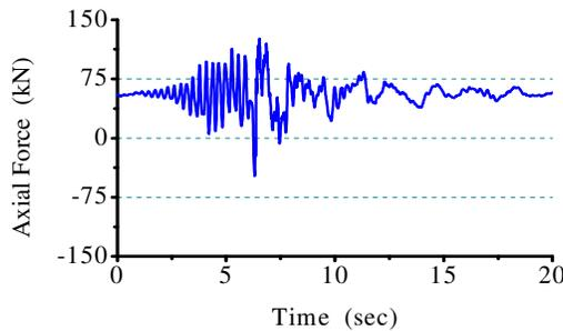
Figure 10. Time history of axial force at bearing (Case-2).
