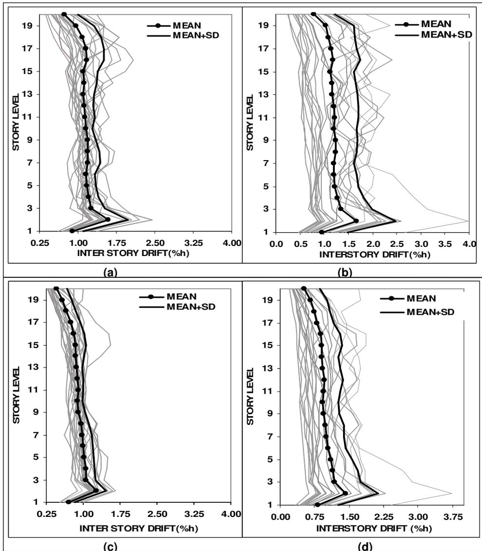
Figure 4. Dynamic analysis for the scaled real ground motion records; (a) bare frame – GM scaled by the “partial area method”, (b) bare frame – GM scaled by the “ordinate method”, (c) infill frame – GM scaled by the “partial area method”, (d) infill frame - GM scaled by the “ordinate method”.
