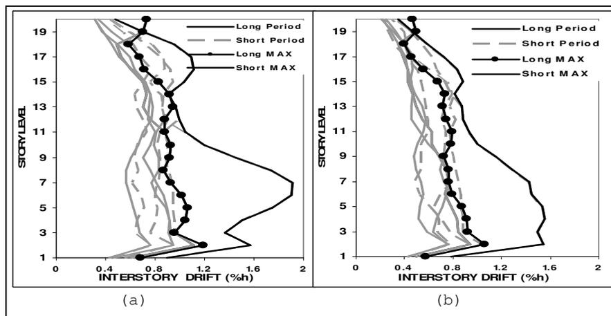
Figure 3. Dynamic Analysis for the Stochastic Ground Motion records (a) bare frame (b) infill frame.
