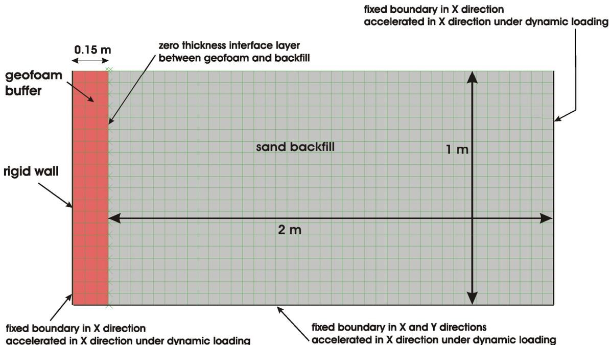
Figure 6. FLAC numerical grid showing geofoam buffer, sand backfill and boundary conditions.
