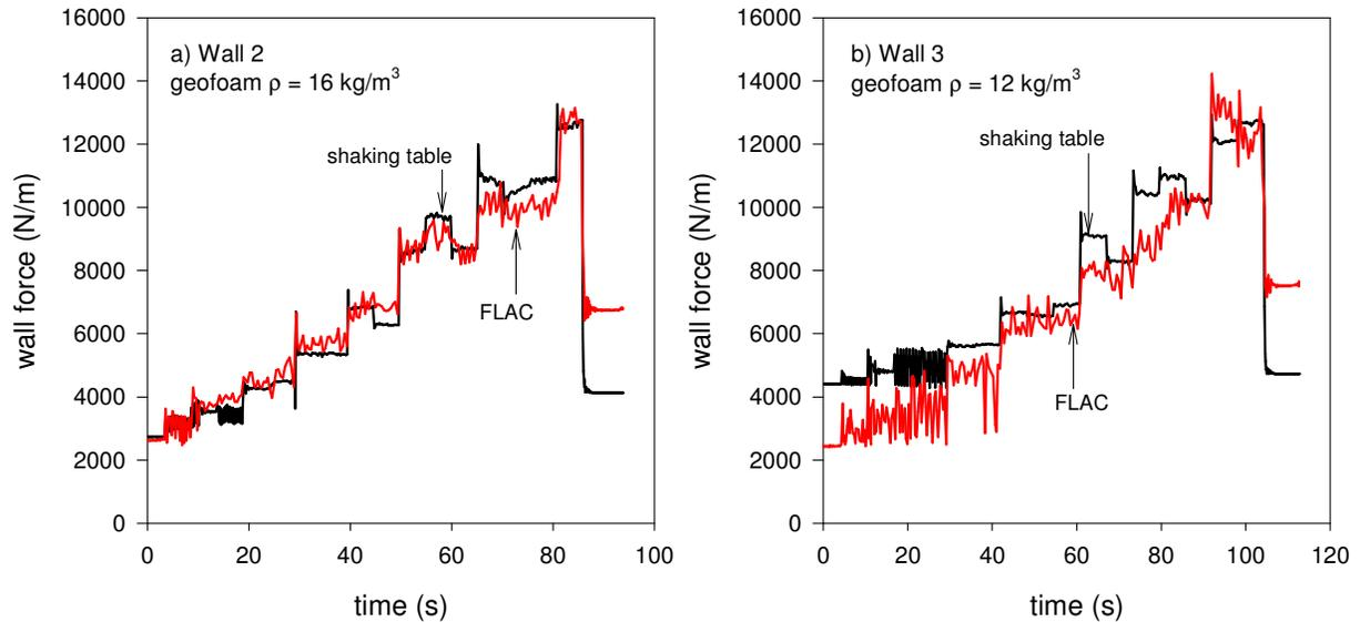
Figure 7. Wall force - time histories from physical tests and FLAC numerical simulations.
