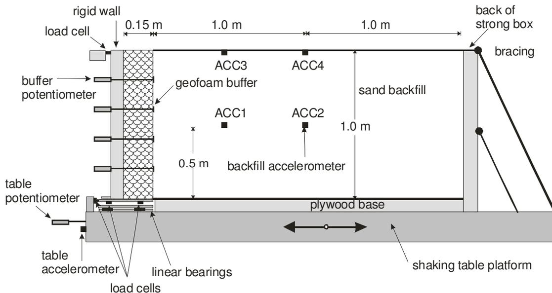
Figure 1. Example shaking table test configuration and instrumentation.
