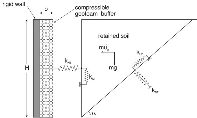
Figure 4. Single block displacement model.
