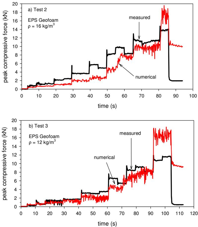
Figure 5. Wall force - time histories from physical tests and simple displacement numerical model.
