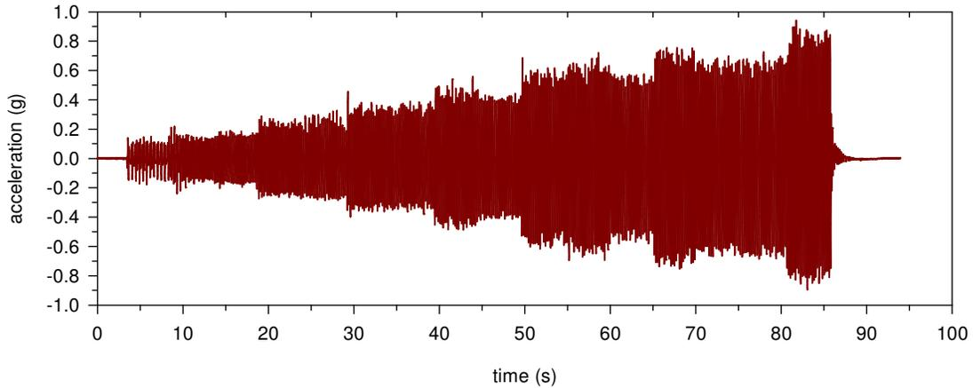
Figure 2. Example measured stepped-amplitude sinusoidal base excitation record – filtered to 12 Hz and linear baseline corrected.
