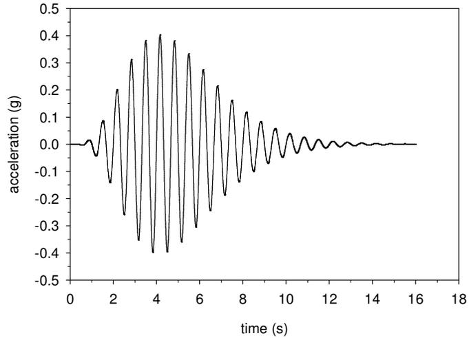
Figure 8. Example input acceleration history for prototype-scale FLAC model with frequency of 1.5 Hz and peak acceleration of 0.4g.
