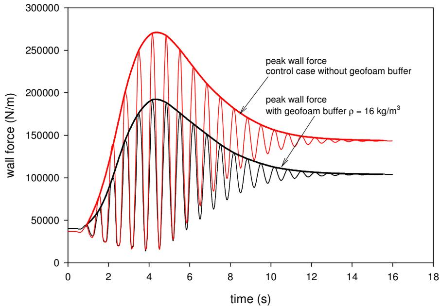
Figure 9. Horizontal wall force variation with time for prototype-scale control wall and wall with seismic buffer.
