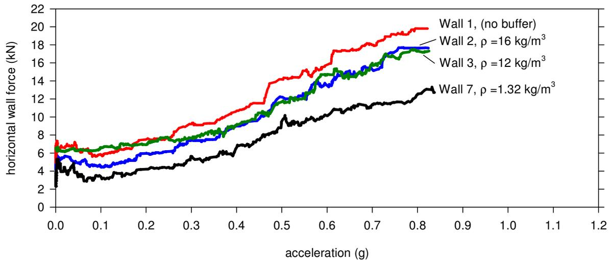
Figure 3. Horizontal wall forces recorded at peak base acceleration amplitude levels for Walls 1, 2, 3 and 7.
