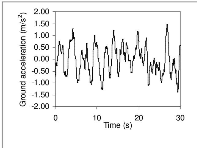
Figure 3. Segment of time history of artificial ground acceleration for which ANNs are trained.
