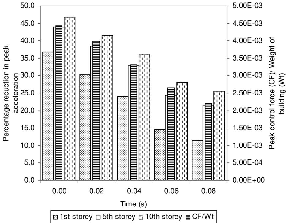
Figure 8b. Acceleration control (target reduction = 50%, three-mode response for Treasure Island).
