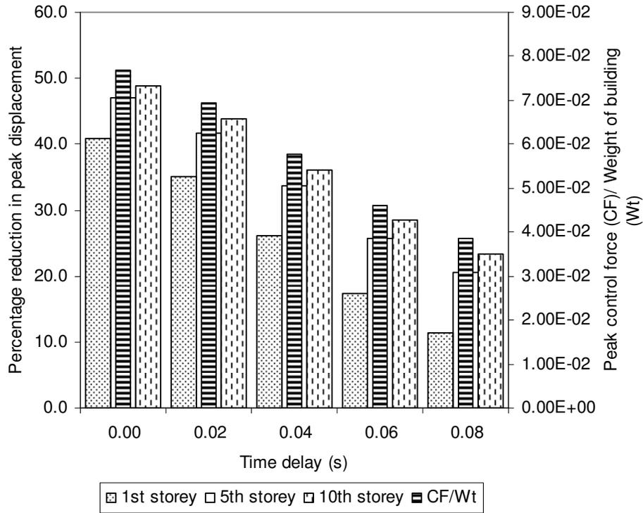
Figure 7a. Displacement control (target reduction=50%, three-mode response for El Centro)
