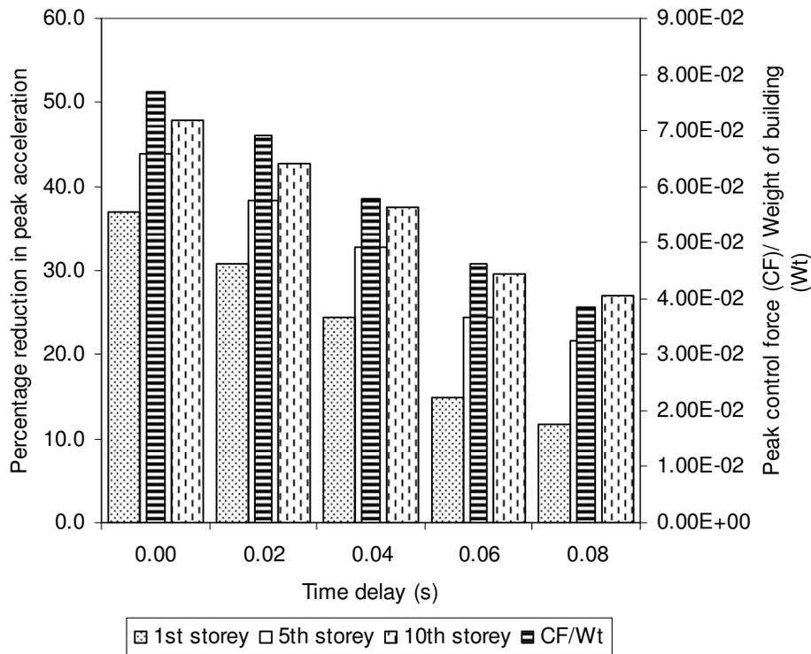
Figure 7b. Acceleration control (target reduction = 50%, three-mode response for El Centro).
