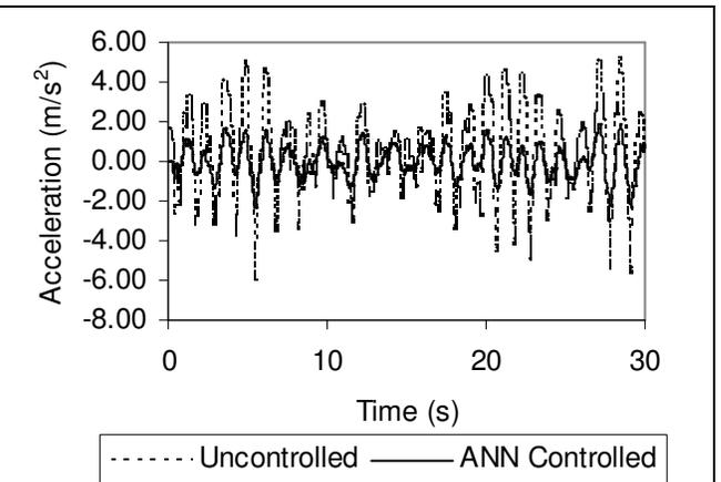
Figure 6. Time history of acceleration for top story (target reduction = 50%).
