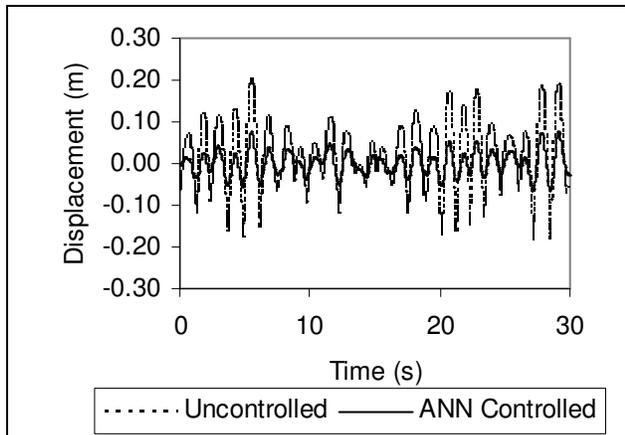
Figure 5. Time history of displacement for top story (target reduction = 50%).
