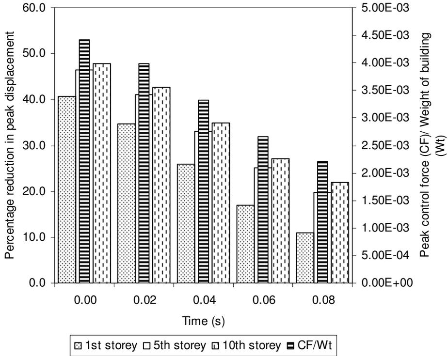
Figure 8a. Displacement control (target reduction=50%, three-mode response for Treasure Island).
