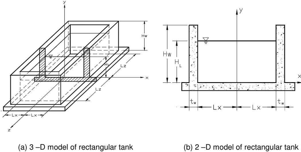
Figure 1. Schematic of rectangular tank.
