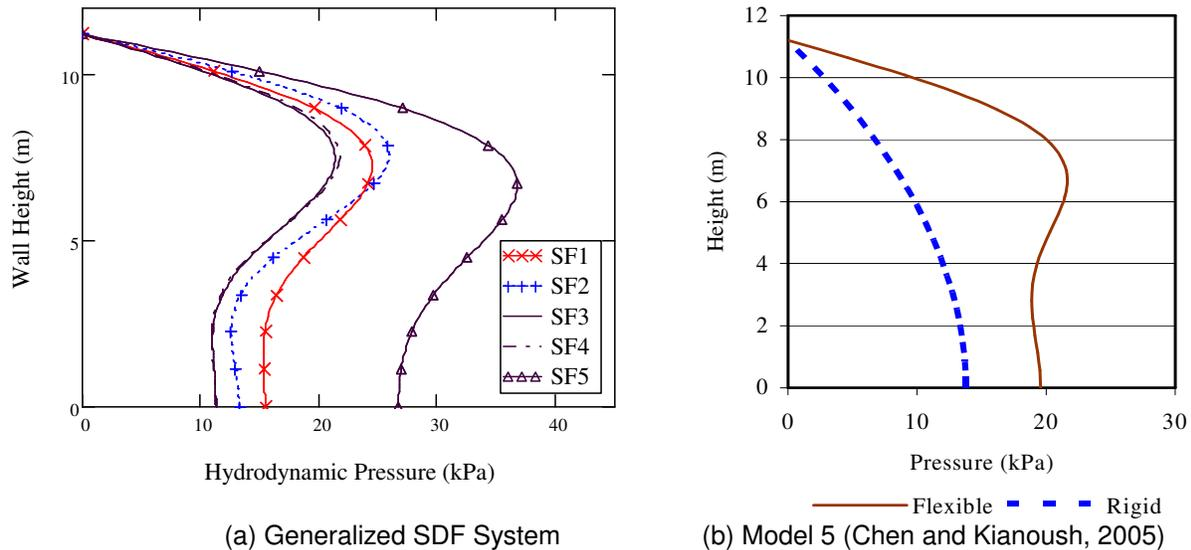
Figure 5. Hydrodynamic Pressures Distribution along Height of Wall.
