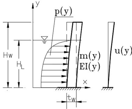
Figure 2. Concrete Rectangular Tank in Generalized SDF System.
