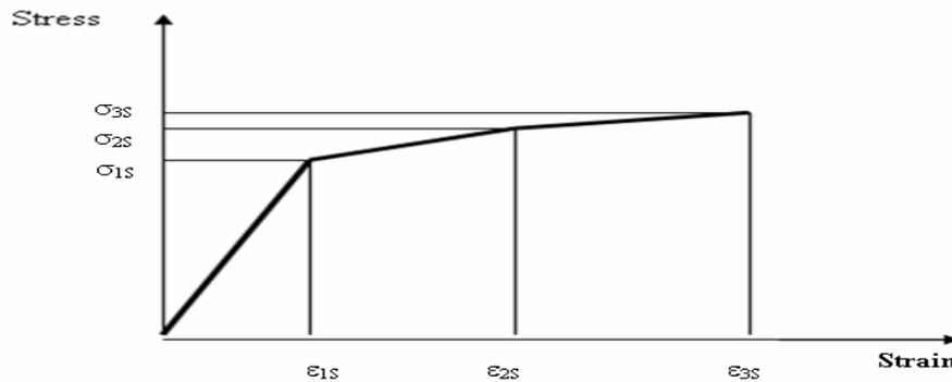
Figure 2. Material model for steel in DRAIN-2DX.
