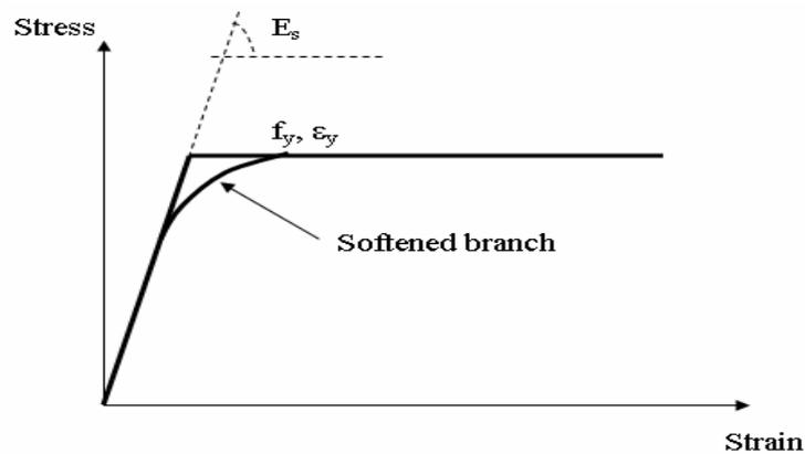
Figure 4. The softened branch in the stress-strain behavior of steel.
