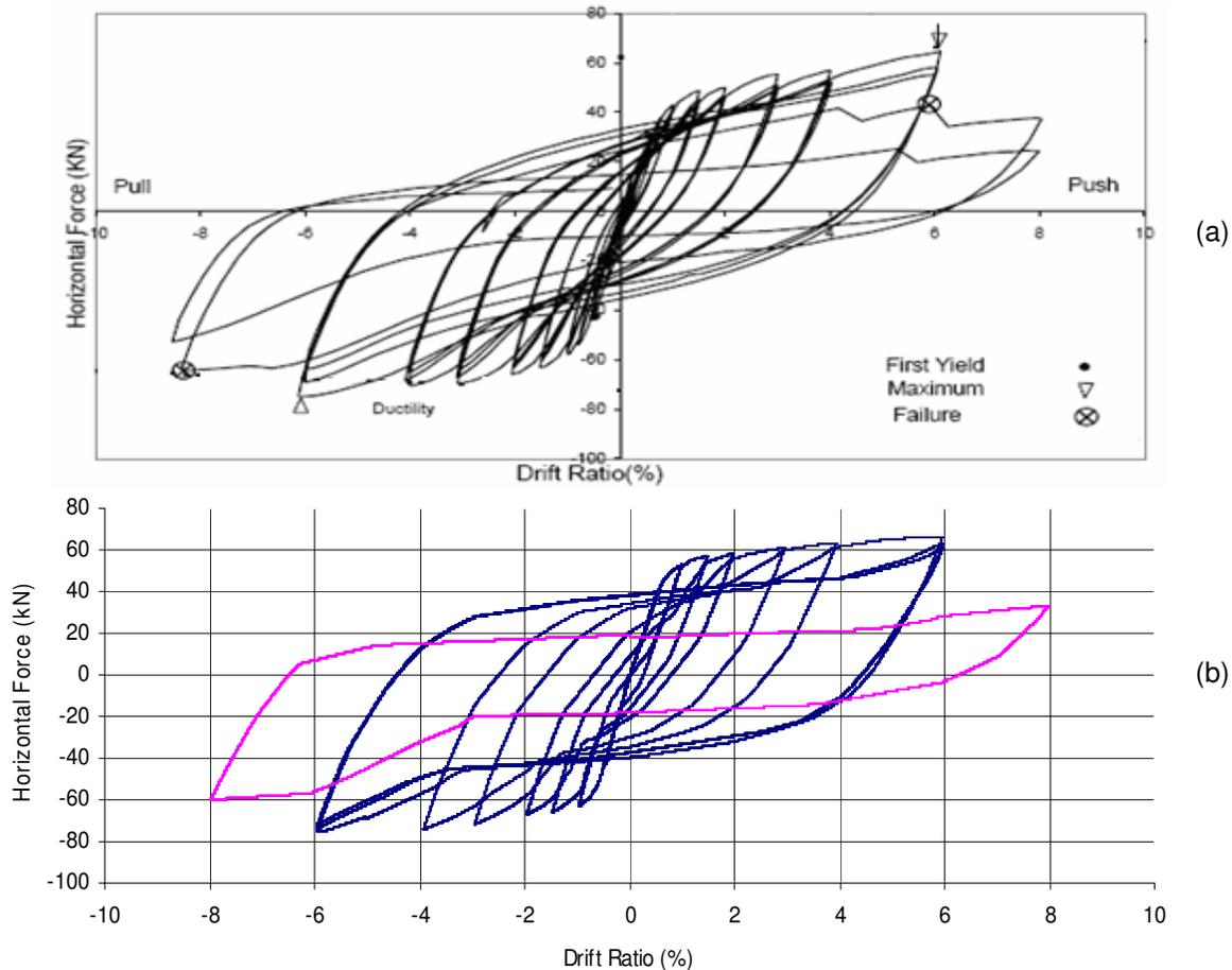
Figure 8. Horizontal force-top displacement response for the column. (a) experimental (Esmaily 1999), (b) trilinear model.
