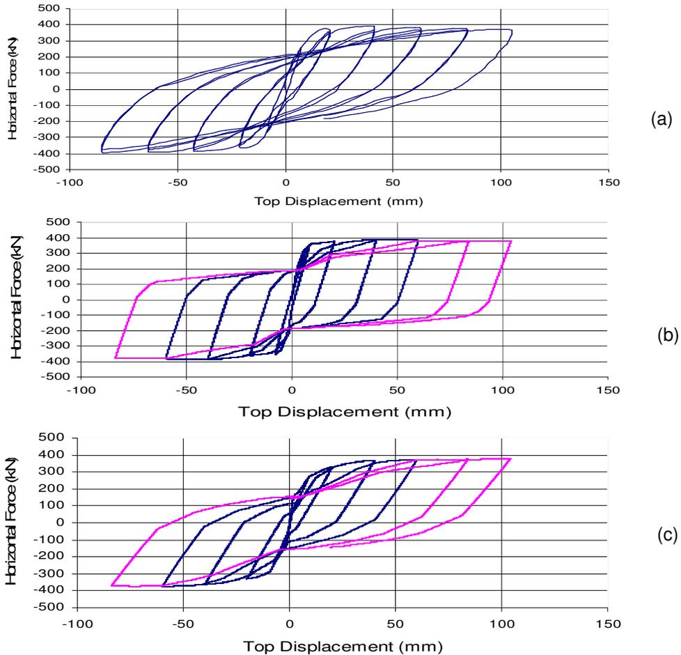
Figure 7. Horizontal force-top displacement response for the column.
