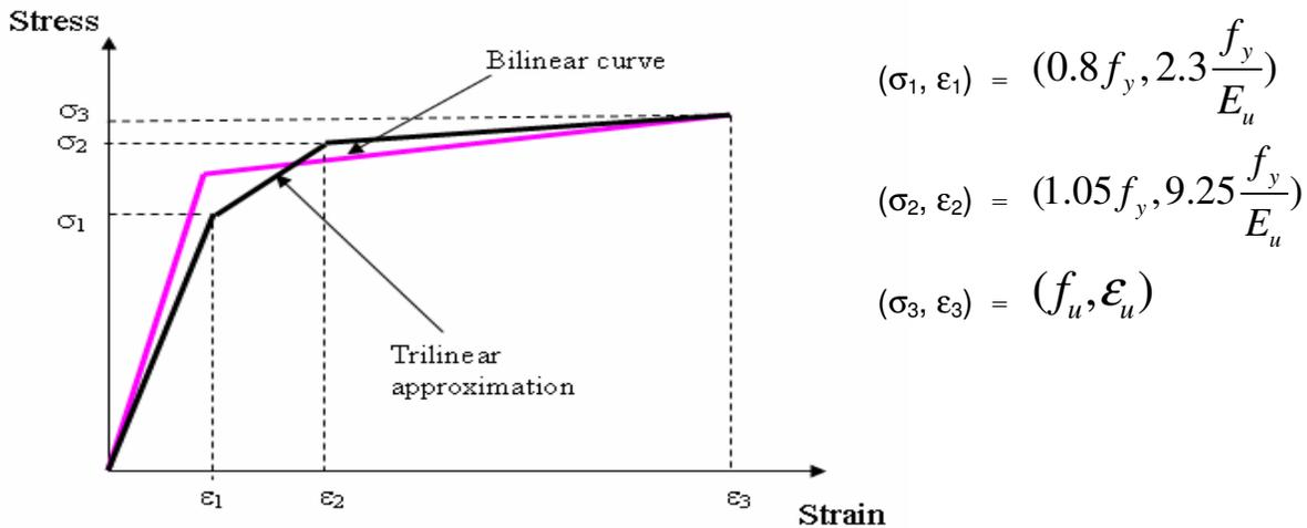
Figure 5. The proposed trilinear material behavior for steel.
