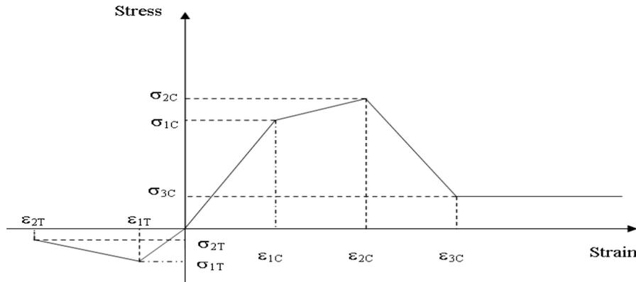
Figure 1. Material model for concrete in DRAIN-2DX.
