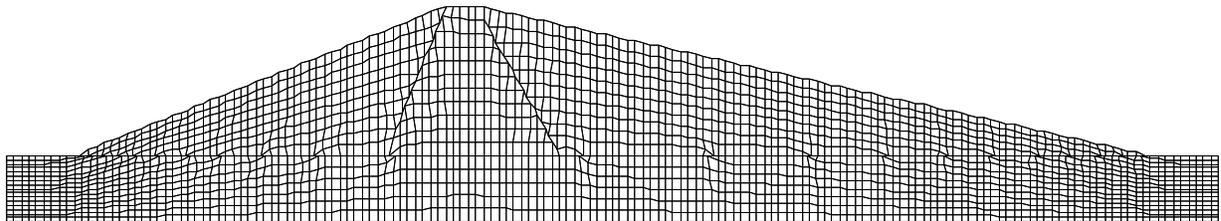
c) 2D model of maximum cross section of the dam
