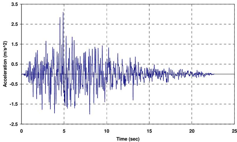
Figure 2. Input acceleration time history developed as rock out crop motion.
