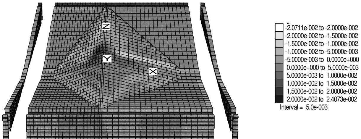
Figure 7. Displacement contours along the dam axis for the 3D analysis.
