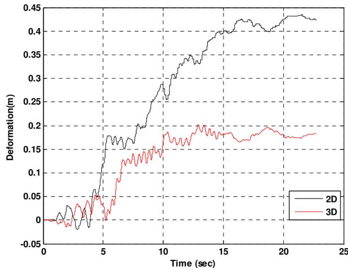
Figure 4. Transverse displacement time history of the dam at the crest.
