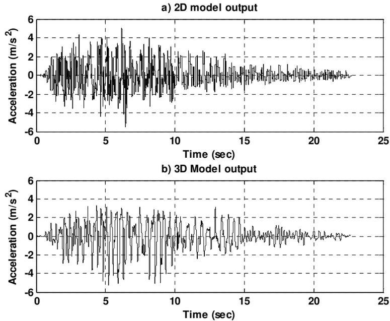
Figure 3. Acceleration time history at crest of the dam monitored at similar locations.
