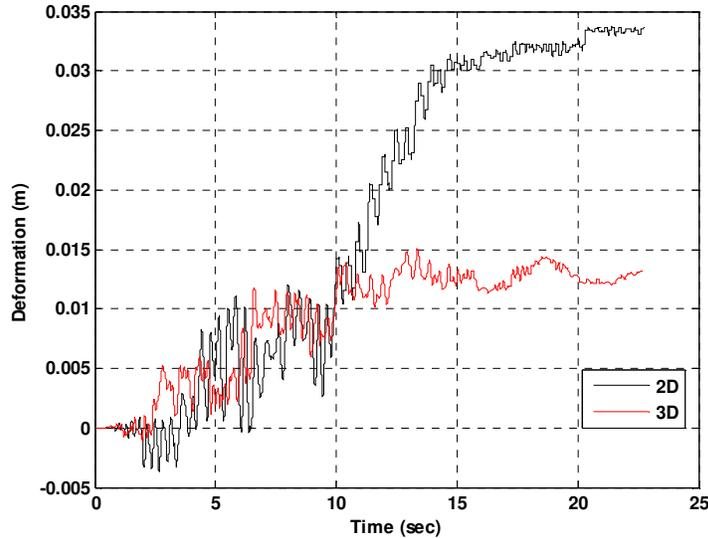
Figure 5. Vertical displacement time history of the dam at the crest.
