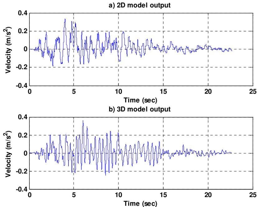
Figure 6. Transverse velocity time history monitored at the crest of the dam.
