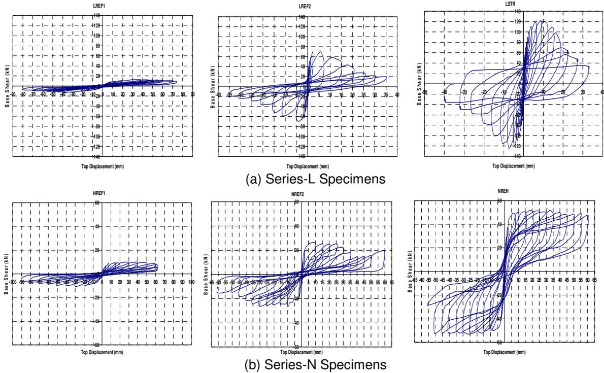
Figure 7. Load-Roof Deflection hysteresis curves of the test specimens.
