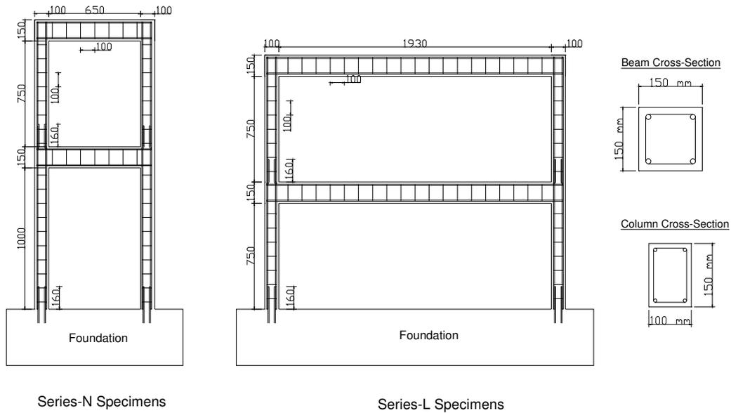
Figure 1. Dimensions and reinforcement details of the test specimens.
