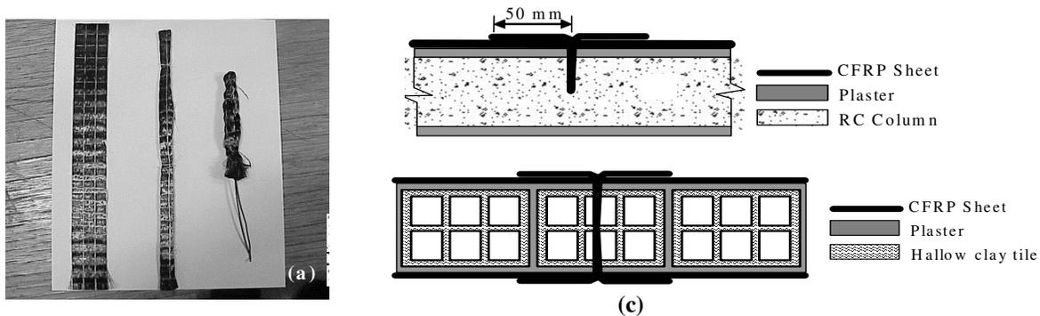
Figure 2. (a) Made-up Anchor dowels; and application of anchor dowels to (b) the frame members and (c) the masonry walls.
