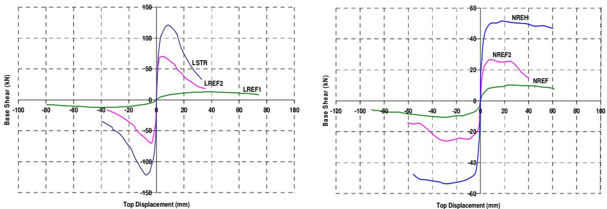
Figure 8. Envelopes base shear-root displacement curves of the test specimens.
