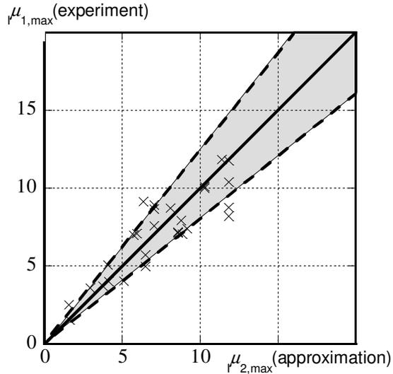
Figure 6. Plastic deformation capacity–plastic deformation capacity of experimental result and approximation at maximum load.
