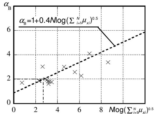
Figure 11. Relationship between cyclic number, amplitude and Bauschinger effect until 95% of maximum load.
