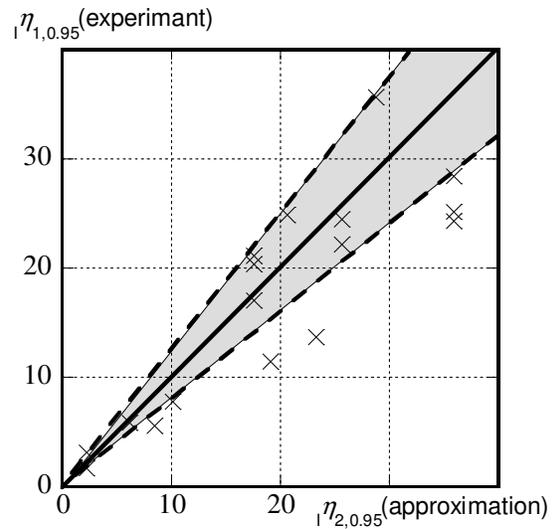
Figure 9. Cumulative hysteresis energy – cumulative hysteresis energy of experimental result and approximation until 95% of maximum load.
