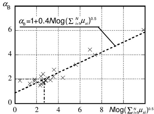
Figure 10. Relationship between cyclic number, amplitude and Bauschinger effect until maximum load.
