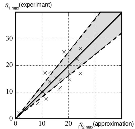
Figure 8. Cumulative hysteresis energy – cumulative hysteresis energy of experimental result and approximation until maximum load
