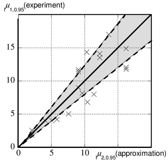
Figure 7. Plastic deformation capacity–plastic deformation capacity of experimental result and approximation at 95% of maximum load.
