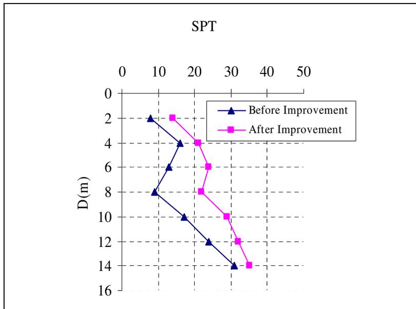
Figure 6. Curve of SPT values at depth of subsoil before and after of improvement.
