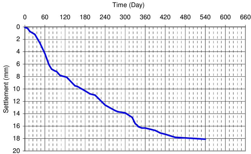
Figure 5. Curve of settlement changes versus time in center of the raft for the Afsoon building project.
