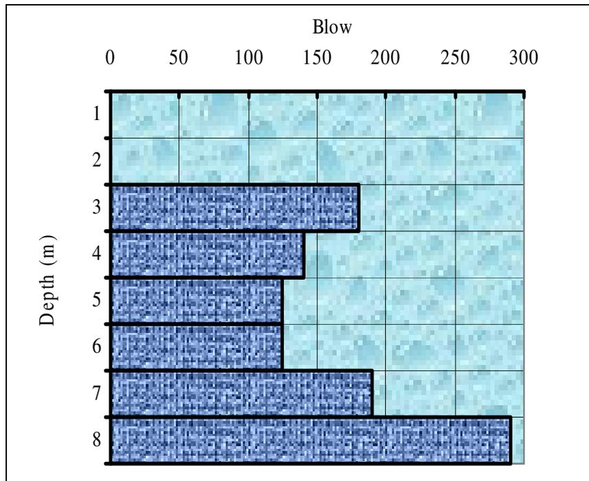
Figure 3. Bearing graph for pile penetration for Test Pile No.12.
