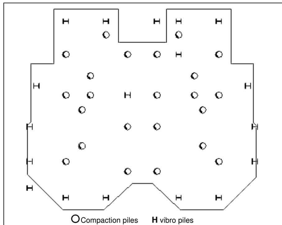
Figure 4. Plan of vibro and compaction piles locations for Afsoon building project.
