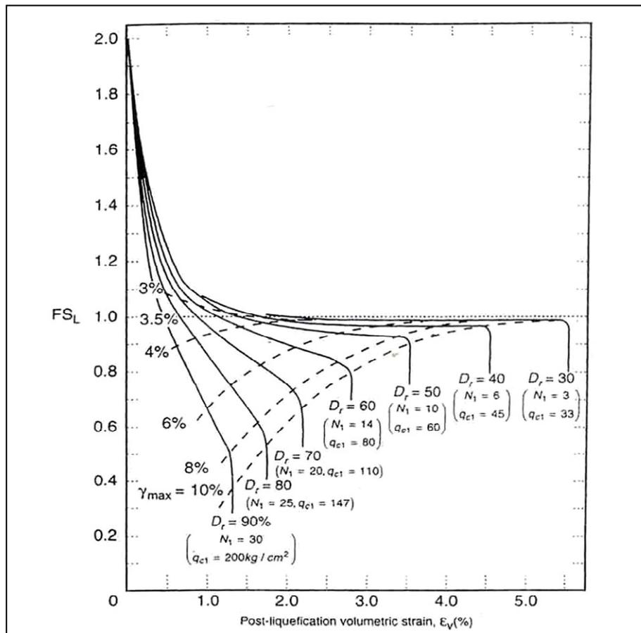
Figure 7. Chart for estimating the ground surface settlement of clean sand as a function of the Factor of Safety against liquefaction (FSL).
