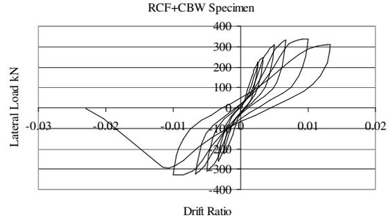
Figure 5. Specimen after failure and test result of top lateral load-drift ratio curve.
