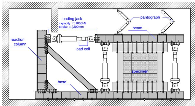
Figure 4. Test and Loading setup of specimen RCF+CBW.
