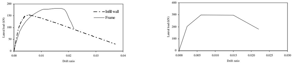
Figure 7. Drift ratio-lateral load response; *Left curve*: Individual response of bare frame and infill wall, *Right curve*: Combined results.
