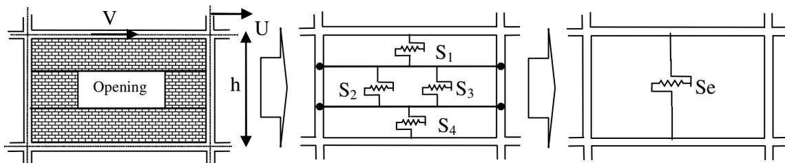
Figure 3. Equivalent spring model for infill masonry walls with openings.
