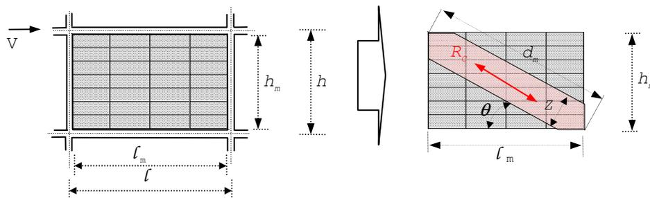
Figure 2. Infill masonry walls and the equivalent diagonal compression strut parameters.
