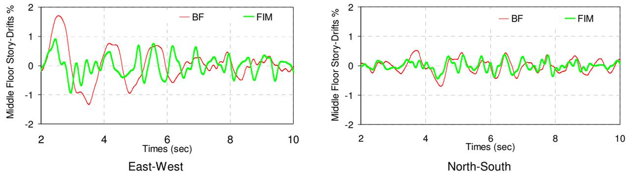
Figure 12. Middle-story drifts ratios (maximum drifts were obtained for this story).
