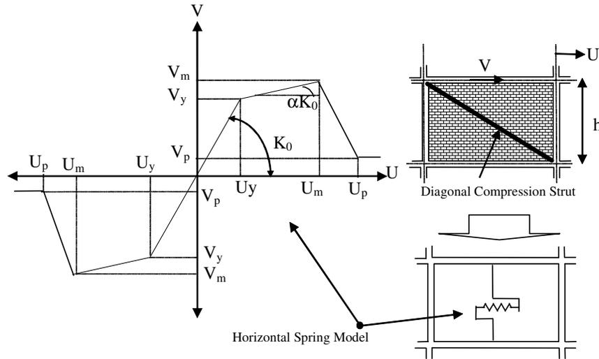
Figure 1. Analytical model for conventional masonry infill walls.
