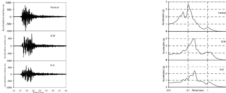
Figure 10. Three components of strong ground motion (left figures) and response spectra (right figure) of the 2003 Bam Earthquake.
