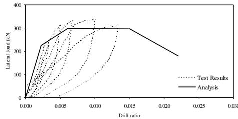
Figure 8. Comparison of test and analytical results for specimen RCF+CBW.
