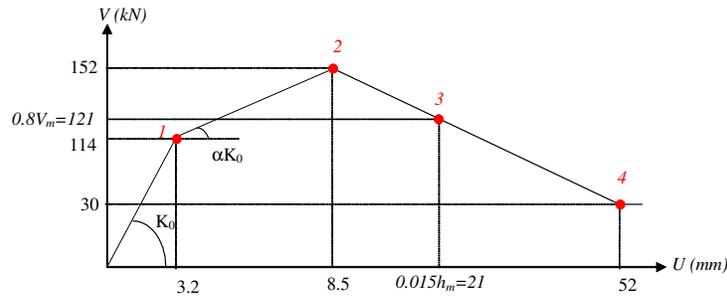
Figure 6. Force-displacement envelope curve for infill wall of specimen RCF-CBW.
