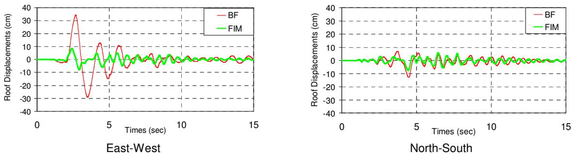
Figure 11. Roof displacement responses.
