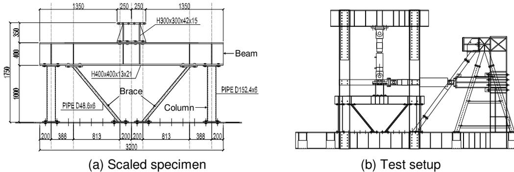
Figure 6. Specimen design and installation.
