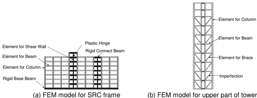
Figure 5. FEM models for numerical substructures.
