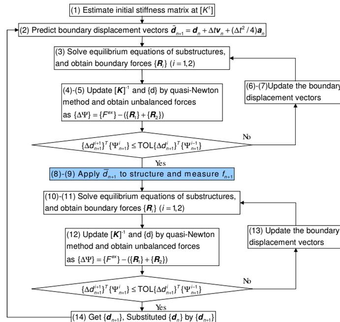
Figure 2. Testing scheme featuring two-round quasi-Newton procedure (Pan 2006).
