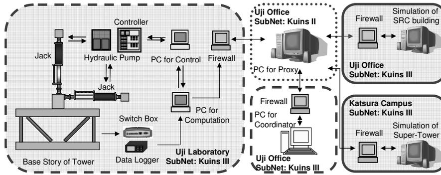
Figure 7. Distributed online hybrid test system.
