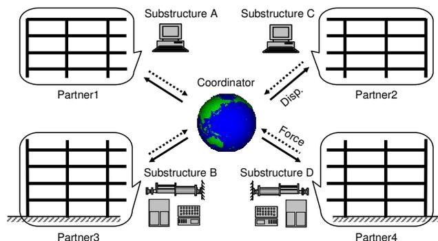
Figure 1. Concept of P2P Internet online hybrid test system (Pan 2006).
