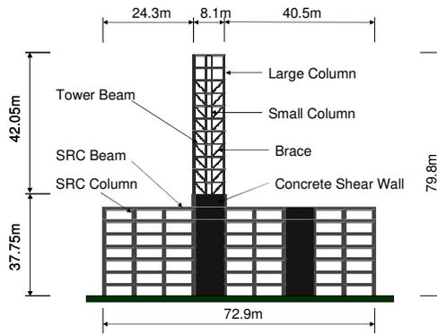
Figure 4. Simplified planar structure.
