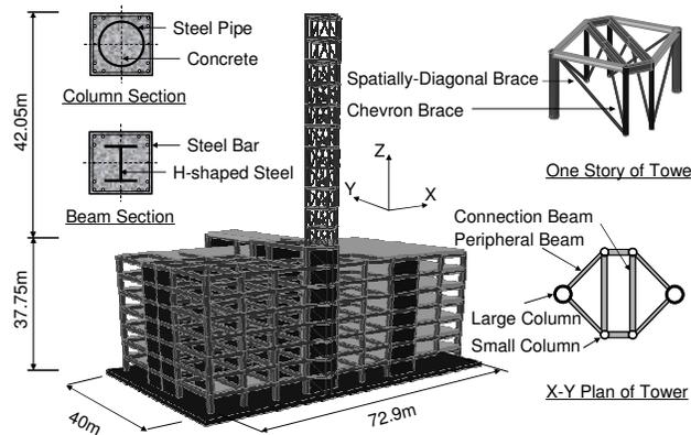
Figure 3. SRC structure with a steel tower.
