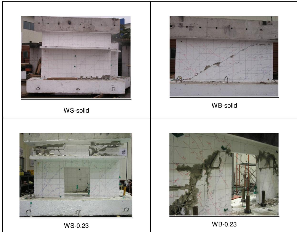
Figure 4. Observed cracks and final failure mode.
