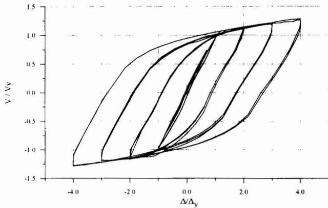
Fig. 4 Load-deformation response of the frame.
