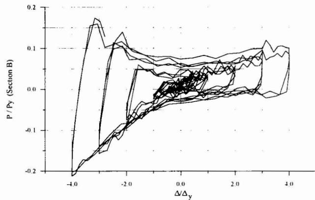
Fig. 5 HSS axial load-frame storey drift (left brace).
