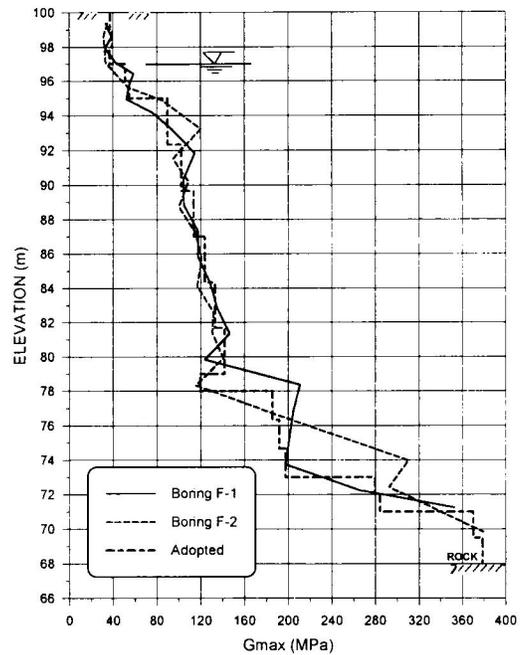
Fig. 8 Shear modulus profile.
