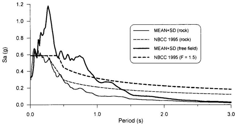
Fig. 7 NBCC and ground motion response spectra.
