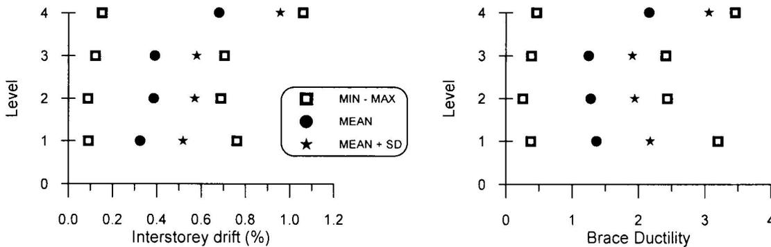
Fig. 9 Results of the analysis: a) peak interstorey drift; b) peak brace ductility demand.
