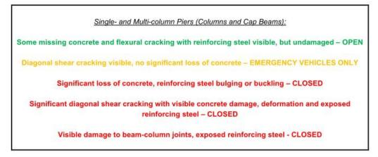
Figure 4. Post-earthquake inspection manual recommendations
