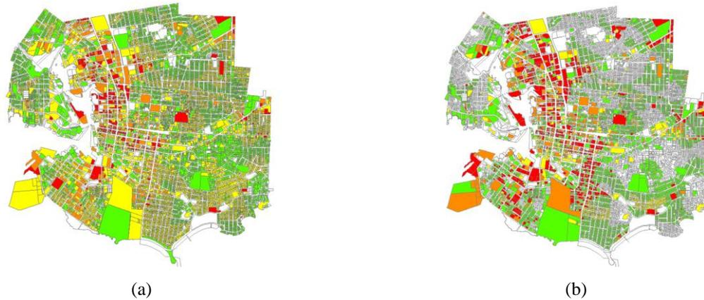
Figure 6: Damage Distribution for the Probable Magnitude = 9 Subduction Scenario (a) HAZUS (b) OpenQuake
