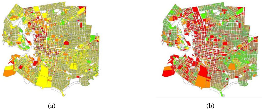
Figure 5: Damage Distribution for the Magnitude = 7 Crustal Scenario from: (a) HAZUS (b) OpenQuake
