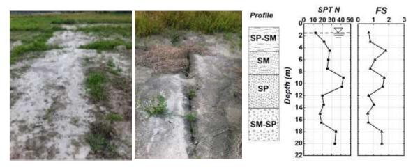
Figure 4 Bungmati: observed liquefaction, soil profile, SPT-N value and factor of safety against liquefaction
