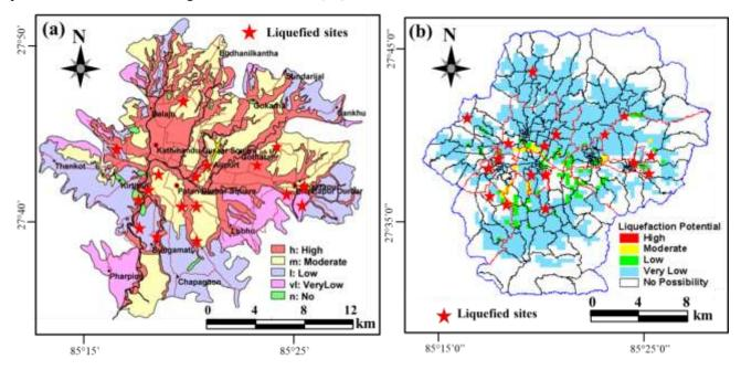
Figure 8. Liquefaction hazard maps with some typical liquefied site during 2015 earthquake (a) UNDP/MOHPP [25] and JICA [26].
