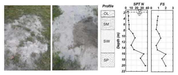
Figure 5 Duwakot: observed liquefaction, soil profile, SPT-N value and factor of safety against liquefaction
