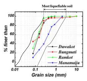
Figure 7. Typical particle size distribution of the soil at some liquefied sites. Range of most liquefiable soil after Tsuchida and Hayashi (1971).
