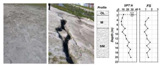
Figure 3 Manamaiju: observed liquefaction, soil profile, SPT-N value and factor of safety against liquefaction
