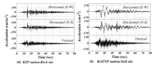
Figure 2. (a) Accelerograms at KTP [20] for the Mw 7.8 main shock, and (b) accelerograms at KATNP for the Mw 7.8 main shock [19]
