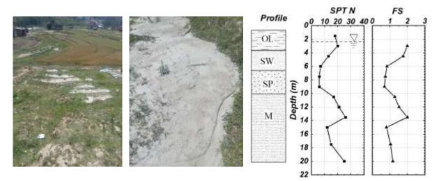
Figure 6. Ramkot: observed liquefaction, soil profile, SPT-N value and factor of safety against liquefaction
