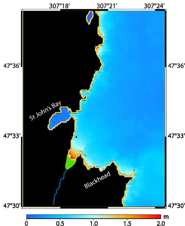
Figure 3. Maximum wave heights on St John's Bay and neighborhood (GR04) after 9 h of tsunami propagation. The green area symbolizes a lagoon system alimeted by a small river and protected by a dune row.
