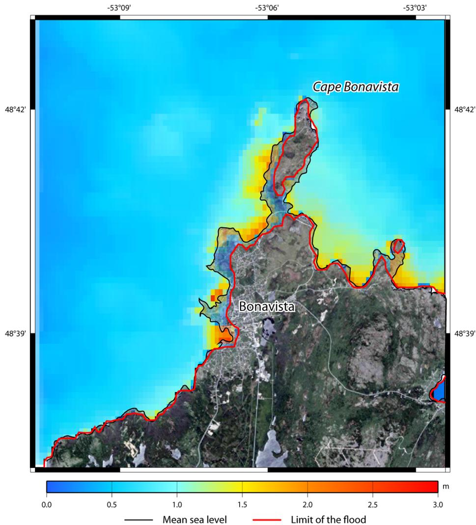
Figure 2. Sea surface elevation and maximum flow depth on the 150 m resolution grid (GR06) showing the Cape of Bonavista after 9 h of tsunami propagation. A satellite view (Google Earth <sup>TM</sup>) allows the correlation between populated areas and wave amplification.
