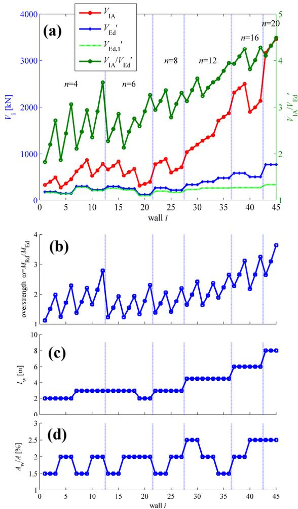
Figure 2: (a) Base shear for the analyzed walls obtained by different methods. The variation of the basic input parameters is shown in Figures (b), (c) and (d).
