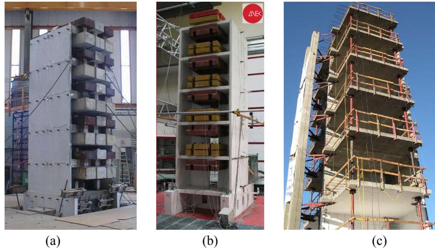
Figure 1. Large-scale models tested on shake-tables (a) CAMUS-3 - Cantilever wall designed according to EC8, (b) ECOLEADER-SLO - Lightly reinforced coupled wall designed according to the Slovenian practice, (c) UC San Diego - Full-scale model of a 7-story building slice.
