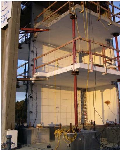
Figure 4. San Diego test setup with gravity columns. Benchmark documentation provided by the UC San Diego; courtesy of Prof. Restrepo.
