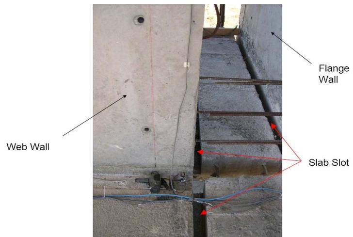
Figure 5. Slotted slab. Benchmark documentation provided by the UC San Diego; courtesy of Prof. Restrepo.
