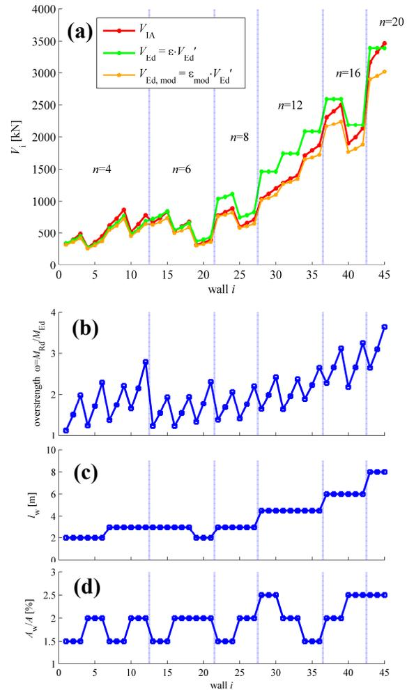
Figure 3: (a) Comparison between the base shear obtained by the EC procedure, modified EC procedure and inelastic response history analysis.
