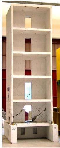
Figure 6. Damage to the ECOLEADER-SLO wall at the end of the test.
