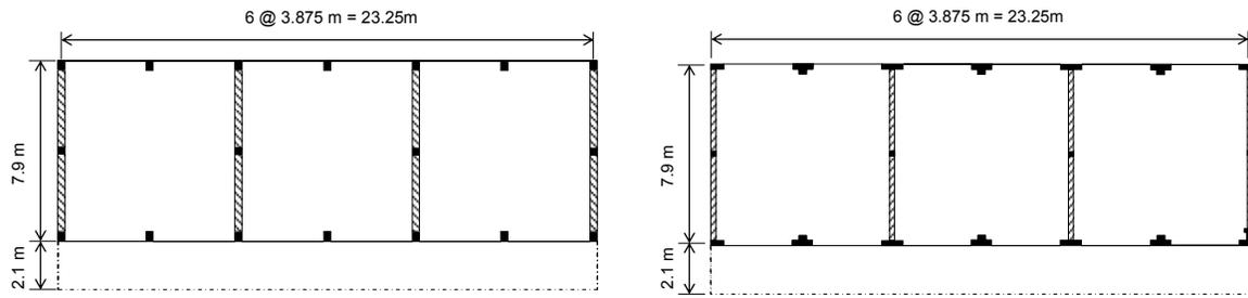
Figure 11. Plan for template school buildings in Peru built per 1977 (left) and 1997 (right) codes. Solid rectangles/squares/T-shapes: columns; hatched: confined masonry walls; solid lines: perimeter masonry infill walls. The 2.1m balcony overhang is also shown.
