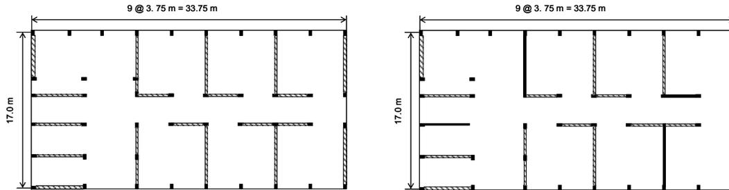
Figure 1. Floor plans for template RC moment-resisting frame (left) and dual system (shear wall and moment-resisting frame) (right) schools in Turkey. Solid small rectangles: columns; solid long rectangles: RC shear walls; hatched long rectangles: full-bay masonry infill walls; solid lines: perimeter masonry infill walls with openings.
