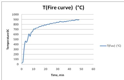
Figure 3: CAN/ULCS101 fire curve
