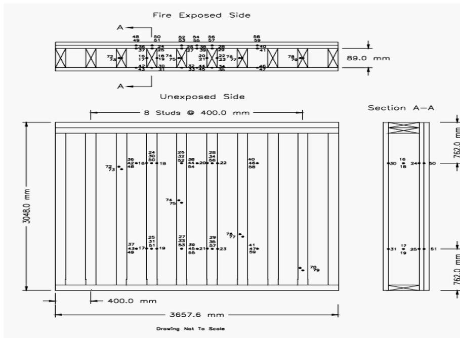
Figure 2: Wood stud assembly F-19, NRC fire test (Kodur and Sultan, 1996)
