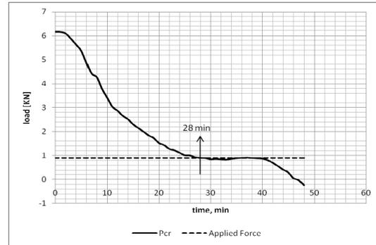
Figure 10: The wood stud wall buckling capacity during PEF and 30% earthquake damage ratio.
