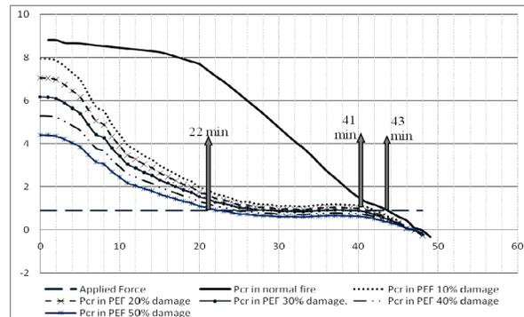
Figure 12: Reduction in the wall buckling capacity due to earthquake
