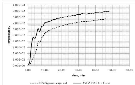
Figure 4: Temperature on the gypsum board
