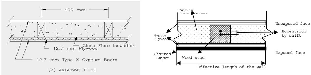
Figure 7: The effective length of the wood stud wall with charred layer
