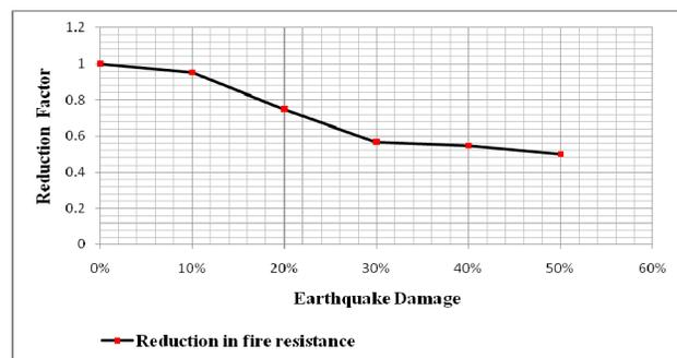
Figure 13: Reduction in fire resistance of the wood shear wall
