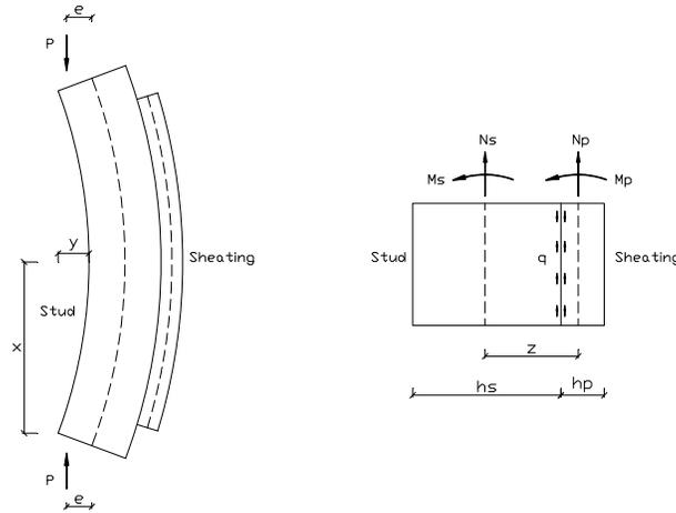
Figure 1: The sheathing to framing buckling model.
