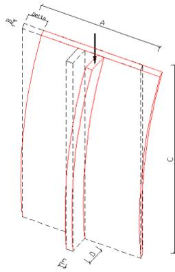
Figure 9: lateral deflection in the wall strip due to earthquake load.
