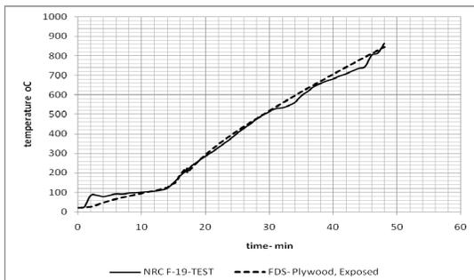
Figure 5: Temperature history results in the plywood layer
