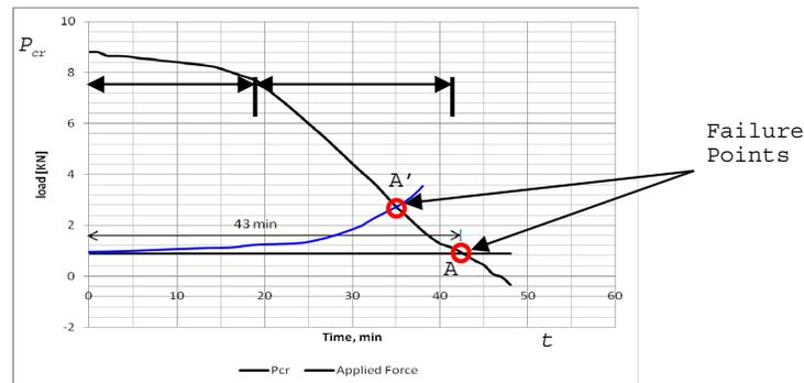
Figure 8: F-19 Buckling capacity degradation with time during fire
