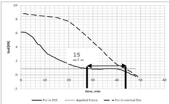
Figure 11: comparison between the wall buckling capacities in fire with and without earthquake (with 30% damage ratio)
