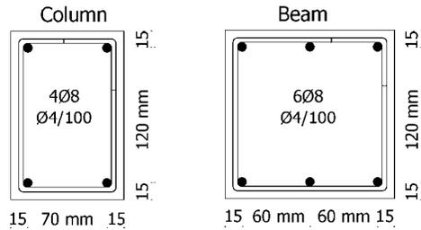
Figure 2. Column and beam reinforcement
