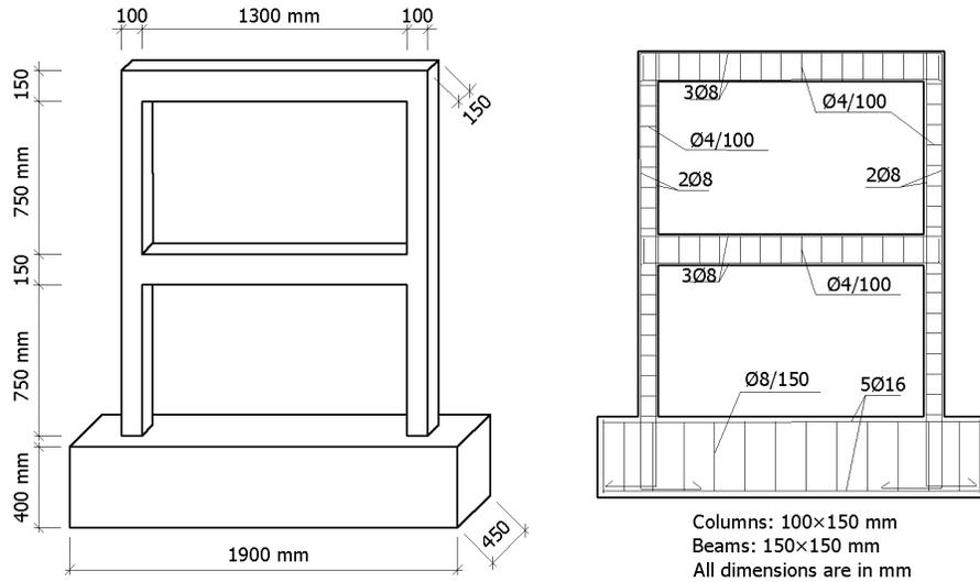
Figure 1. Dimensions and reinforcement patterns of the test specimens
