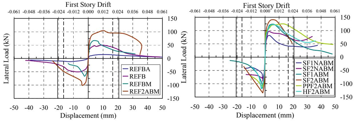
Figure 5. First story envelope graph of specimens
