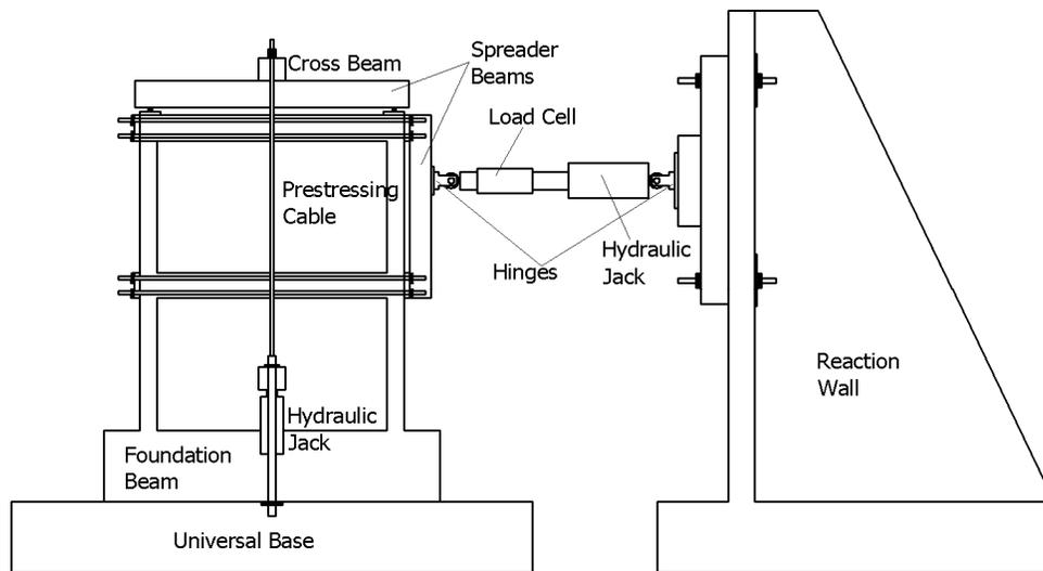
Figure 3. Test set-up
