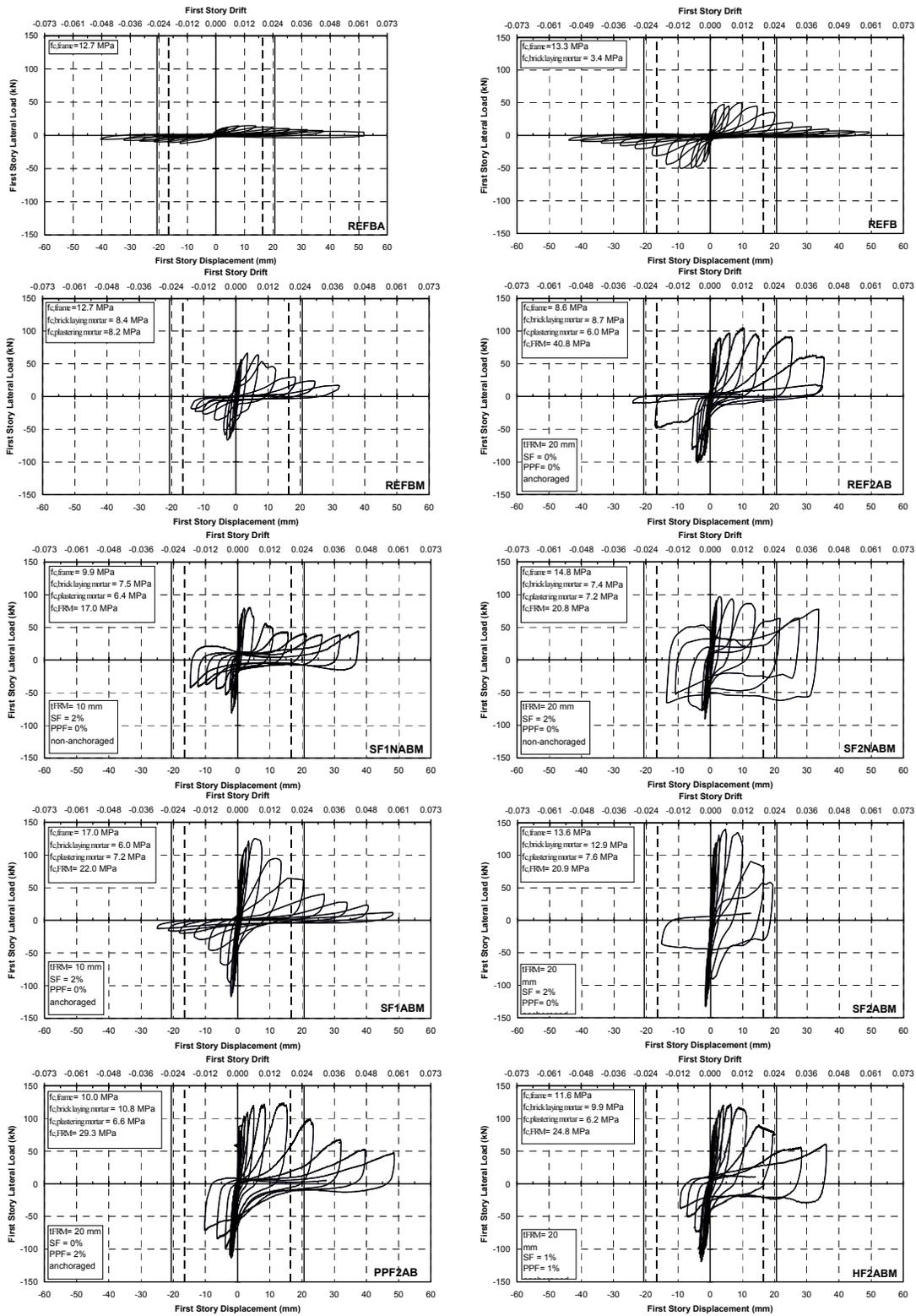
Figure 4. First story lateral load-first story inter-story displacement/drift graphs of the specimens
