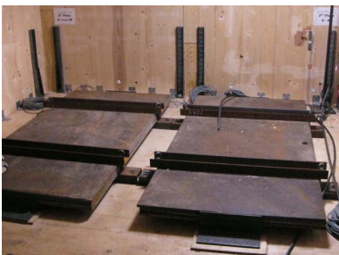
Figure 8. Additional load on floor In Europe, X-lam buildings are usually very heavy. Due to acoustical insulation, an extra layer of sand and a floating floor is added. Furthermore, the tested buildings was not finished, but consisted only of the wooden elements. Therefore, additional loading has to account for the heavy floors, insulation and other wall finishing as well as for 30% percent of imposed loads as required by (Eurocode 0). The three-storey building was additionally loaded as shown in Fig. 8 with 15t per storey; the seven-storey building with 30t per storey. In total, the three-storey building weighed 465kN whereof 30kN additional load. The seven-storey building had a total weight of 2840kN whereof 1500kN additional loading.
