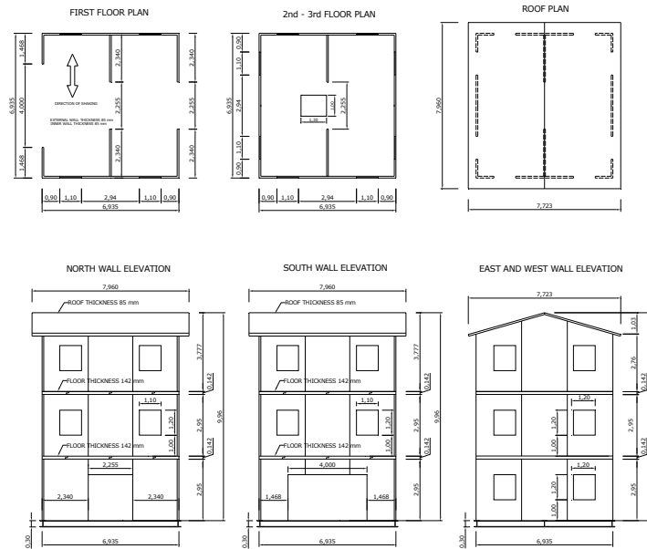
Figure 3. Plan views and elevations of three-storey building in configuration C
