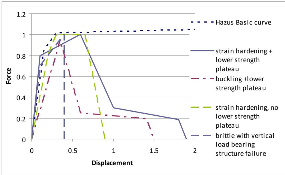
Figure 2. Idealised curves for structural types with different postpeak behaviour.
