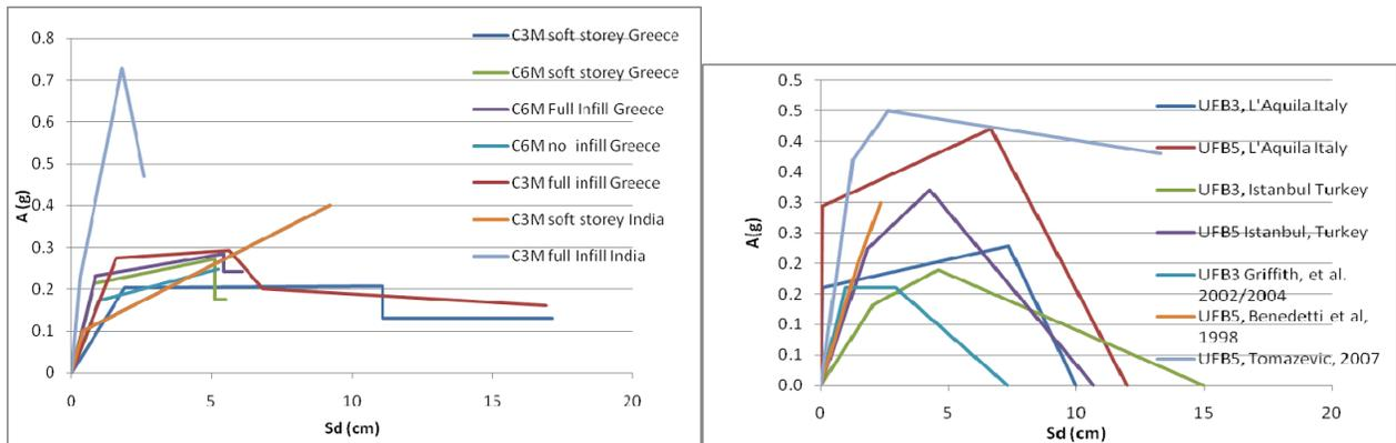
Figure 3. Push-over/capacity curves a) non ductile concrete frames and dual system for Greece and India, b) unreinforced fired-brick masonry in lime mortar without and with concrete slabs and comparison with experimental references.
