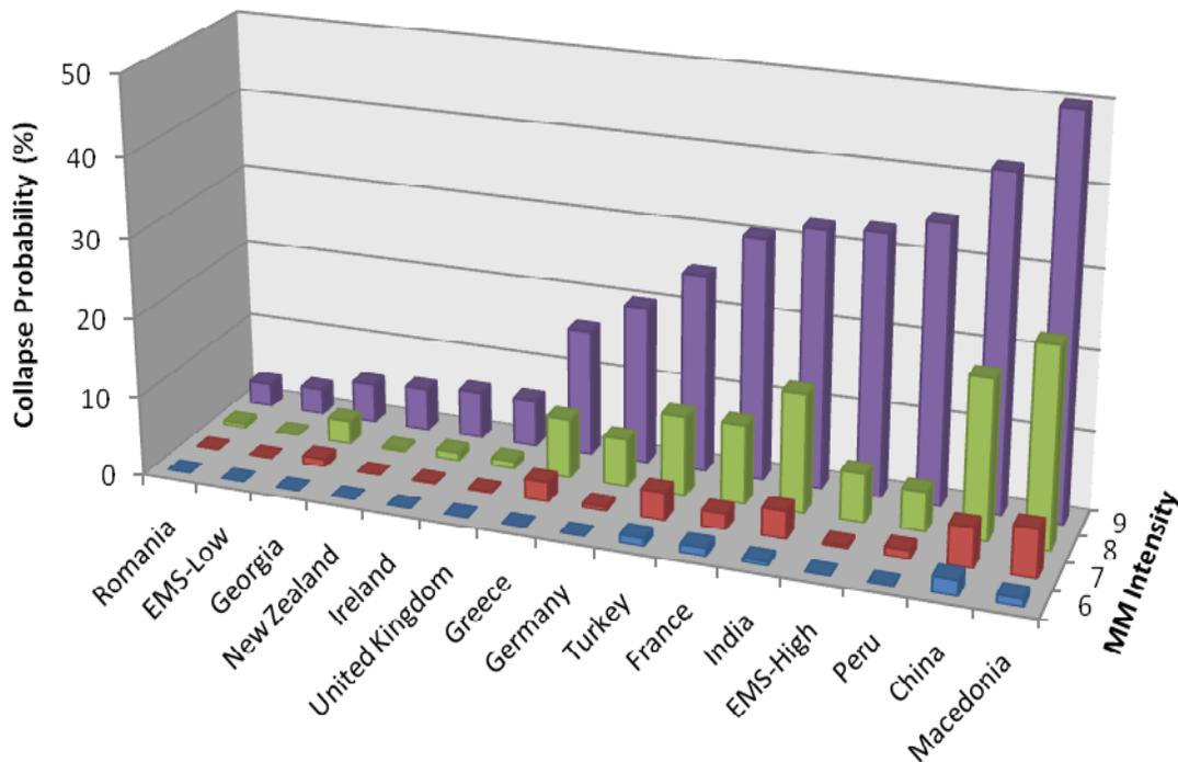
Figure 1. Expert judgment/empirical collapse fragility and expected range of EMS based collapse fragility for unreinforced fired-brick masonry in cement mortar.
