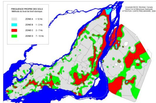
Figure 6. Soil fundamental frequencies for Montreal and the South Shore.
