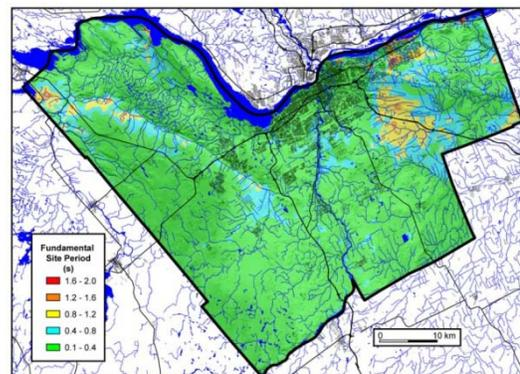
Figure 5. Map depicting ranges of the fundamental site period of the ground within the city of Ottawa area. See text for how fundamental site period was calculated.
