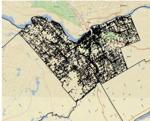
Figure 4. Map showing the location of ~21,000 water well and engineering boreholes in the greater Ottawa area.
