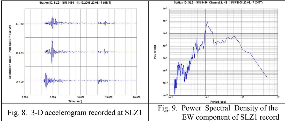
Fig. 8. 3-D accelerogram recorded at SLZ1
