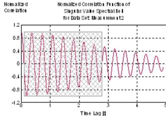
Figure 5b. The corresponding damped vibration of a SDF system
