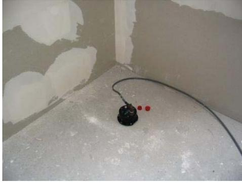
(a) tri-axial sensor in node 1
