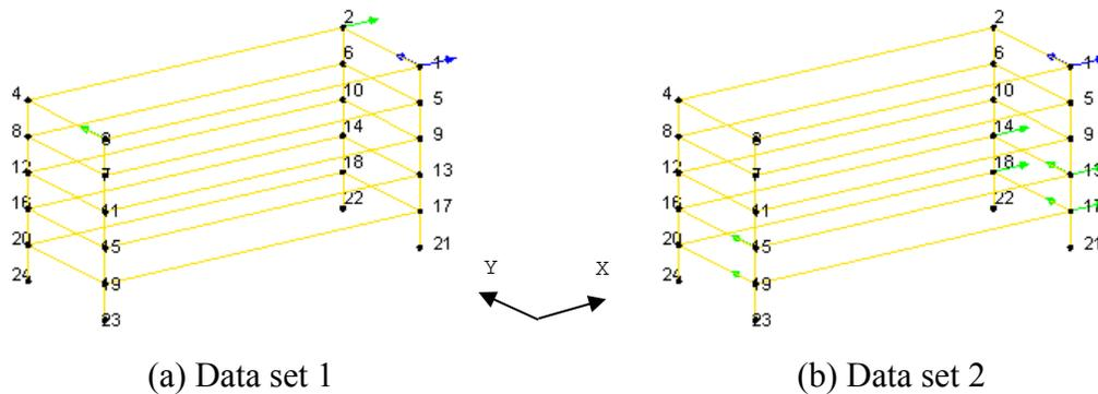
Figure 1. Disposition of sensors by data sets
