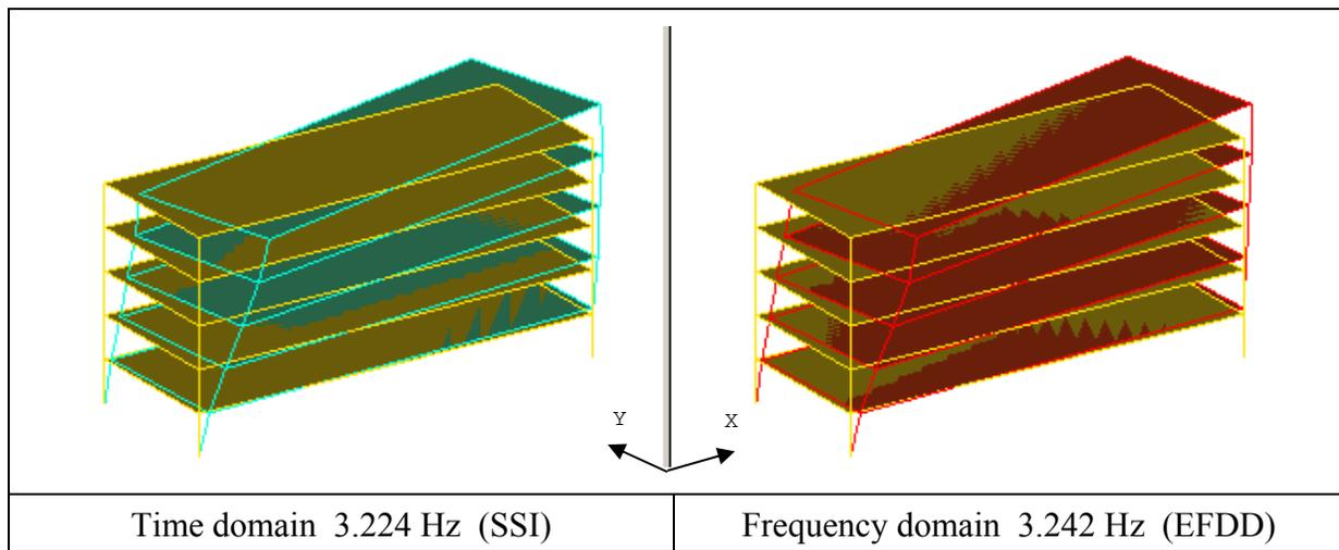
Figure 6. Visualizations of the 2-nd mode shape obtained by the SSI and EFDD methods
