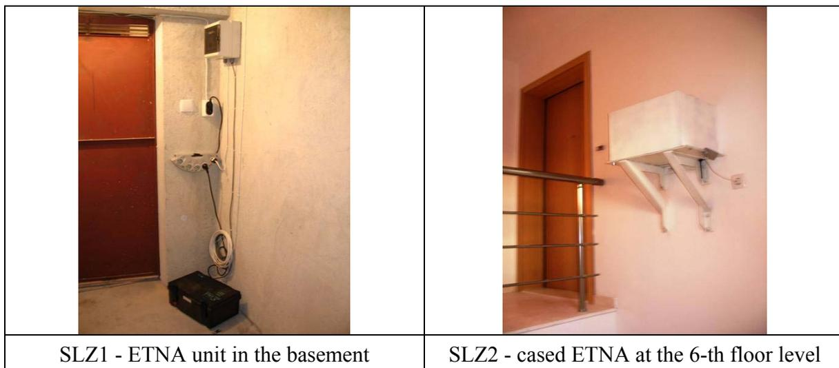
Figure 7. Permanent seismic instrumentation in RC building
