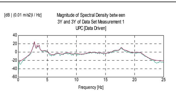
Figure 4. Comparison of the spectral densities for data set 1, sensor 3Y
